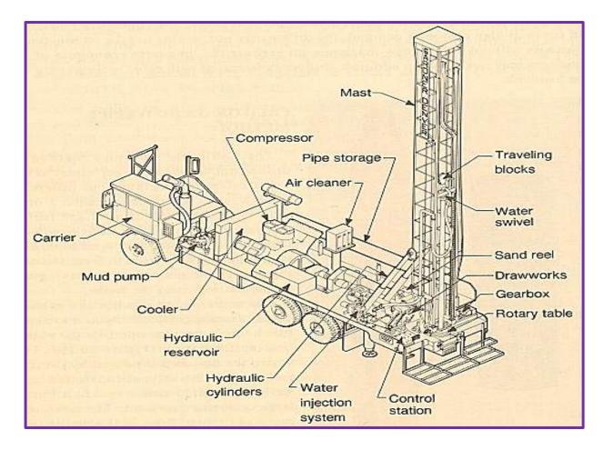
**1. Prime Movers:** The prime movers in a rotary drilling are the driving systems that provide energy power to an entire rig. Generally, steam engines supplied power to the early drill rigs, but currently gas and diesel engines connected with generators, became a standard after World War II. Natural gas or steam is commonly used in reciprocating turbines, which also generate electricity to provide incidental lighting, pumping water, and air compression requirements for the wellsite.
