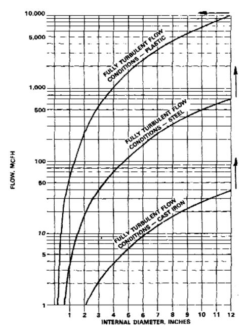
BASED UPON: IGT DISTRIBUTION EQUATION AND FULLY TURBULENT EQUATION, K=0.01 in. FOR CAST IRON, K=0.0007 FOR STEEL. K=0.00006 FOR PLASTIC, K=0.00006 CENTIPOISE.
