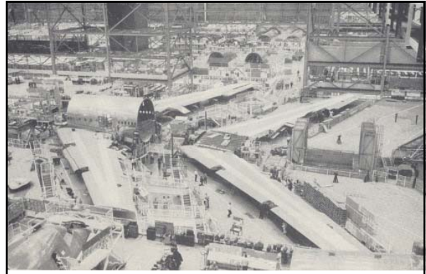
Above: caption: "Wing-body join station precedes joining of the three main fuselage sections at the next station. Station shown is in one of two final assembly bays in use. A third bay is used for subassembly work." 446
