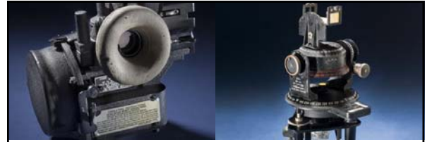
Left: caption: "Mark V Sextant." This averaging sextant was reliable and accurate but heavy (used mainly by the Navy). The hook allowed the navigator to hang the bulky sextant from the top of an astrodome for more precise readings.
