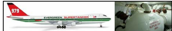
Evergreen Aviation converted two 747s into a "Supertanker" configuration for fighting forest fires. Modifications included:
