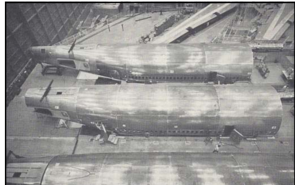
Above: caption: "Aft fuselage consists of Northrop section 46 and LTV section 48. Section 48 comprises the forward two-thirds portion and section 46 the tapered rearward part. Each section is assembled from panels from subcontractors into one tube section in jigs. 444 Outline of individual panels can be seen."
