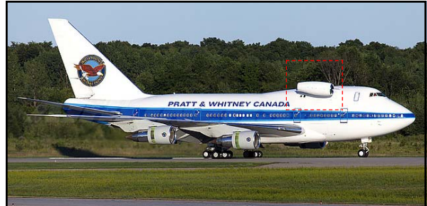
"...Pratt & Whitney's flying test bed is a Boeing 747SP. P&W Canada is in the process of testing their PW1200G engine, that is slated to for the Mitsubishi Regional Jet (MRJ)...P&W uses a Boeing 747SP that was originally delivered to Korean Airlines on January 30, 1980. It flew with the airline until it was placed into storage in 1998. Then in 2008, P&W purchased the 747SP to use for engine testing..." 844 AirlineReporter, May 2012
