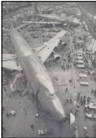
Left: caption: "Overview of final assembly bay shows number two flight test aircraft in last of three assembly and installation positions. Second position was not occupied. Aircraft at top is in final body join. Canting in three final assembly positions helps to utilize space. They are moved on their own landing gear, which can be swiveled." 453
