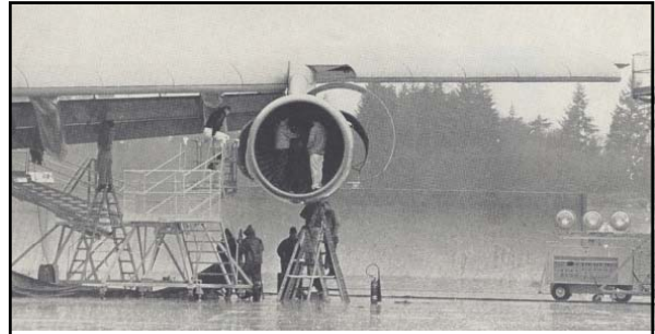
Above: caption: "Ground crewmen give No. 1 Boeing 747 transport prototype Pratt & Whitney JT9D-1 turbofan engine a thorough check at Paine Field, Everett, Wash., after aircraft's first flight. Note size of men in 96-inch-diameter duct." 464
