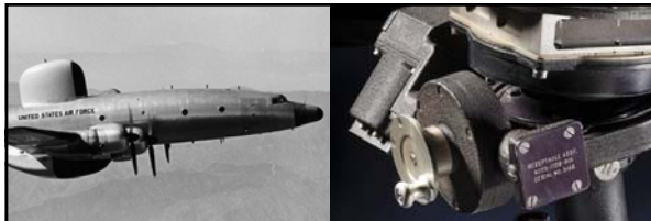
Left: caption: "Lockheed RC-121D." Navigators on civilian airliners and long-range military aircraft, such as the Lockheed RC-121D , began using retractable periscopic sextants in the late 1940s. They eliminated the risk of astrodome blowouts in pressurized aircraft and produced less drag. But their narrow field of view made finding a particular star more difficult.
