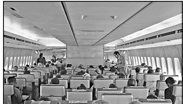
“...As our passenger heads for his seat he'll notice that there are two lengthwise aisles and five cross aisles. Both aisles and seats are at least 10 per cent wider than those on existing 707s. Ceiling height is 8 ft. and walls are near-vertical...”
