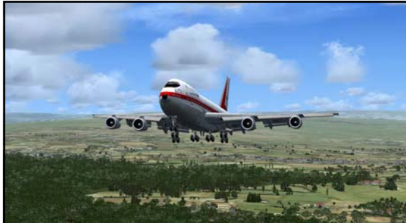
"...When the 747 is in its nose-up landing position, the pilot's eye level will be 37 to 39 feet above the wheel trucks. When the nosewheel is down on the ground, he will still be 28 feet or so above the ground, depending on how much the struts are extended. But these problems are not considered to be serious..." 193 Popular Science, December 1969
