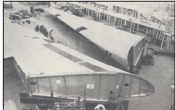
Above: caption: "Each wing, weighing approximately 28,000 lb., then is placed on supports for easier access to finishing. Wing thickness at the root is over 6 ft. Holes in wing leading edges at upper right are for landing lights." 436
