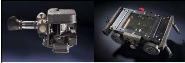
Left: caption: "A-10A Sextant." The compact A-10 was one of the most commonly used sextants in the USAAF. Tens of thousands were made during World War II and many remained in service with the USAF through the 1950s. Key features include a lighted bubble and a recording disk to determine averages.
