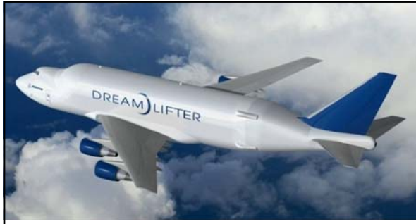
Three Dreamlifters were built (Evergreen Aviation Technologies Corp. of Taipei, Taiwan - a Boeing partner, performed the modifications) and the first trials began in early 2007. Other than the changes to the airframe, the aircraft did not receive any serious modifications (i.e. latest engines and/or avionics) and the modified fuselage was built out of standard aircraft aluminum, not composite materials.
