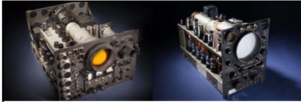
Left: "Western Electric AN/APS-2E Radar Plan Position Indicator." This Navy radar scope would have been used on long-range patrol aircraft, such as the Consolidated PB4Y, late in WWII and during the early Cold War. U.S. bombers during WWII used radar for short-range navigation (under 50 miles) and for bombing through clouds and at night (but less accurately than conventional bombsights). The system was only effective in locating cities and shorelines.
