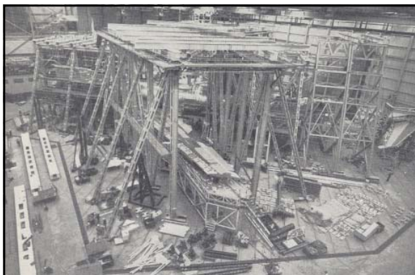
Above: caption: "Static test framework surrounds structurally complete test aircraft. Static tests, including proof pressurization checks began in March. Horizontal stabilizer is tested separately at far right." 455
