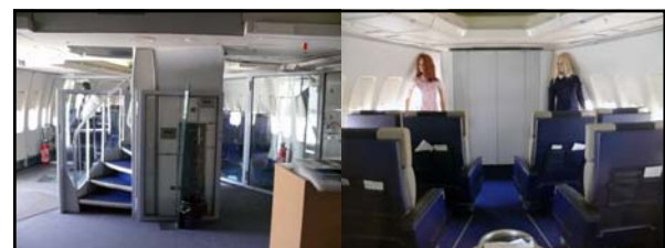
6) FIRST CLASS SEATS Because the fuselage of the B747 tapers toward the nose, the seating configuration of the forward section is quite original. Seats are arranged two by two on each side of the central aisle, in front of the spiral stairway leading to the lounge bar. There are 36 spacious and comfortable seats in First Class, all of them arranged in pairs. 528
