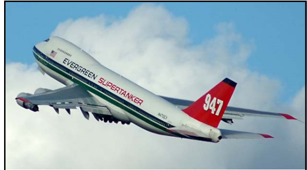
Initial flight of the first Supertanker (a converted 747-200) was in 2004, followed by a 747-100 conversion. Initial operational use was in 2009. After the treacherous 2012 fire season and the loss of several air tankers, the U.S. Forest Service has been providing funding for updating of the U.S. air tanker fleet, the plan being to acquire a number of 747 or DC-10 supertankers as part of the inventory. 842 Above: caption: "Evergreen 747 Supertanker"
