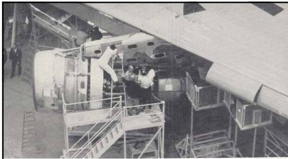
Above: caption: "Workmen check controls of Pratt & Whitney JT9D engine at final assembly and installation position number three on second flight test aircraft. This third final assembly position is last prior to rollout from the factory to the paint hanger. Variable-camber leading edge flaps are at lower right." 449
