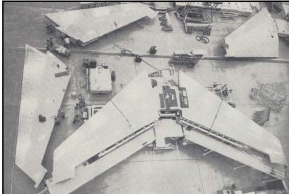
Above: caption: "Horizontal tail is built much the same as the main wing, with each stabilizer attached to a carry-through section to form a single unit. Elevators are installed after stabilizers are mounted to rear fuselage." 451
