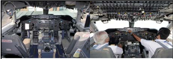
"...The cockpit, which occupies part of a short top deck, bristles with electronic gear, about $1 million worth (a complete plane, if you're in the market, costs about $20 million). In addition to such more familiar equipment as radar scope, radio compass, autopilot, altimeter and so on, the 747 is the first plane to have an inertial guidance system (INS) as standard equipment..." Popular Mechanics, December 1969 Left: caption: "Flight deck displays seen in the Boeing 747 during its Paris Show visit gave little evidence of radically new position display techniques. Control panels and readouts for the Carousel inertial system are situated on the console, while DME readouts are on the left of the co-pilot's panel." Right: caption: "Co-pilot adjusts the INS mode selector in flight" 591
