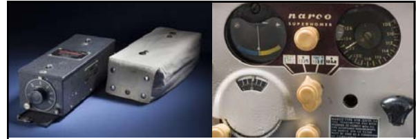
Left: caption: "ZB-1 Radio Homing Adapter and Security Cover." A significant wartime innovation for naval aviators was the YE-ZB radio system, which enabled aviators to find their aircraft carrier without giving away its position. The ship broadcast Morse Code letters in 30-degree arcs. The aircrew flew a heading assigned to the letter. The signals were modulated so they would sound like static if heard without the ZB-1.
