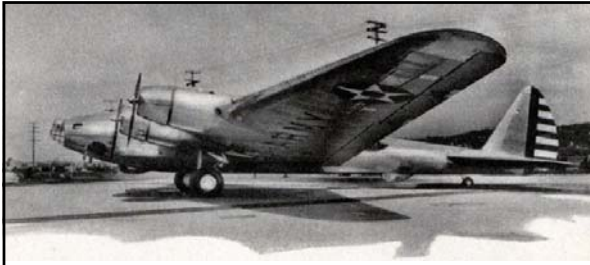
"...Popularly known as the 'flying fortress' this bomber ranked as the fastest and longest range bombardment craft in the world and the largest land plane in America until superseded by the XB-15, a four-engine bomber with a 150-foot wingspan. Designated by the Army as the YB-17, thirteen of these giant planes were ordered by the Air Corps..."
