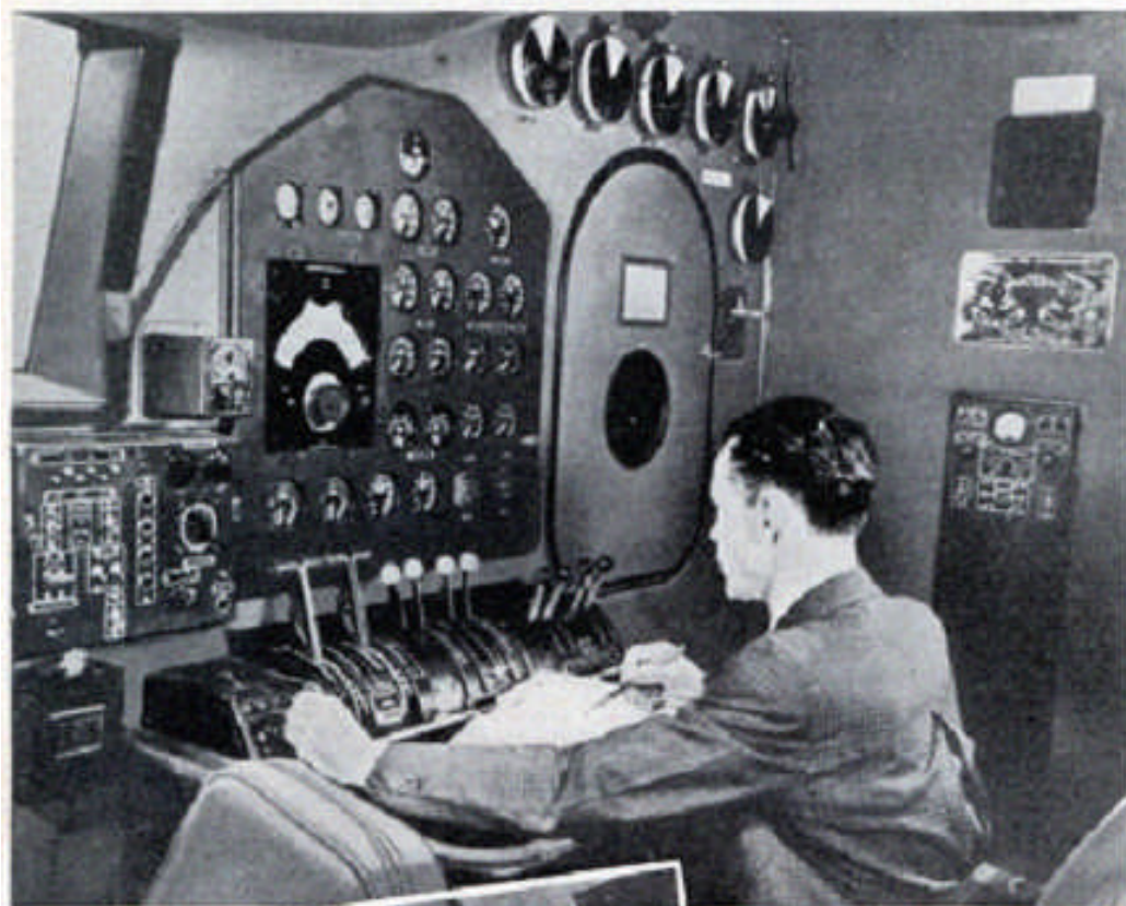
Above: caption: "At this big panel, the flight engineer controls the motors. The door at right leads to a motor-inspection passageway."
