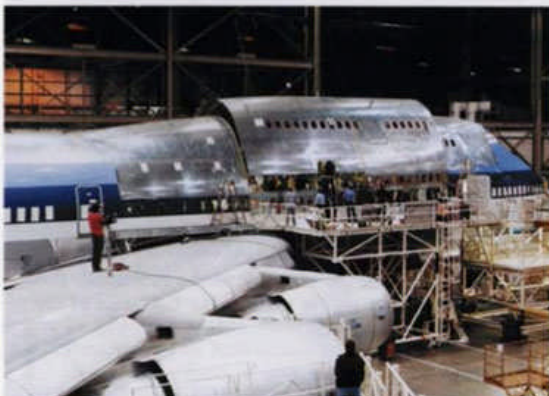
E. New structure positioned.
