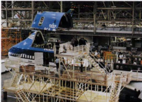
C. Cab crown removed.
