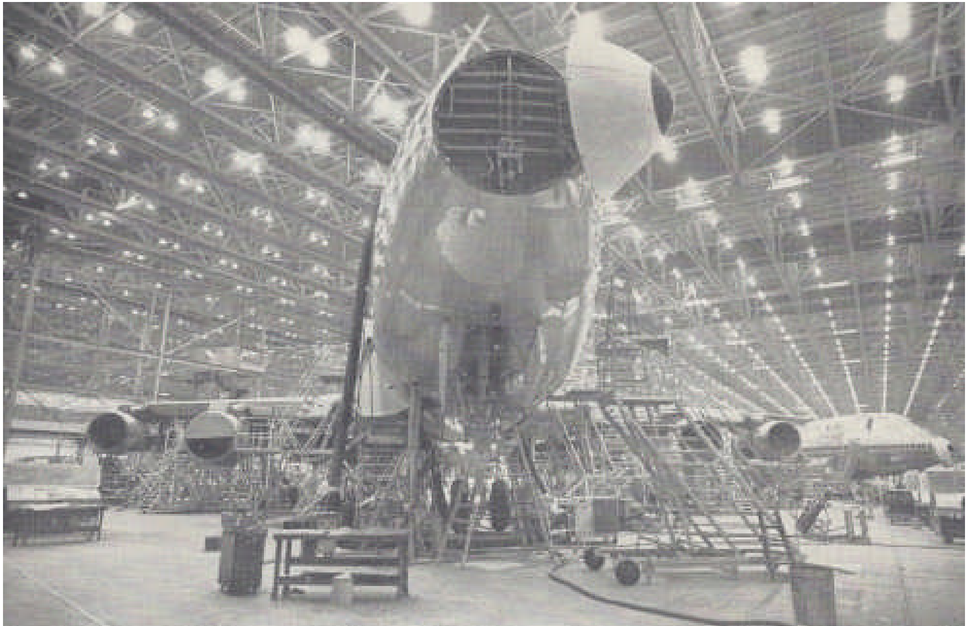
Above: caption: “Ground view of number two 747 in final assembly shows radome swung aside. Aircraft at this point, just prior to rolling out the door, is being subjected to final proof testing of all systems and a structural shakedown of the entire aircraft.”
