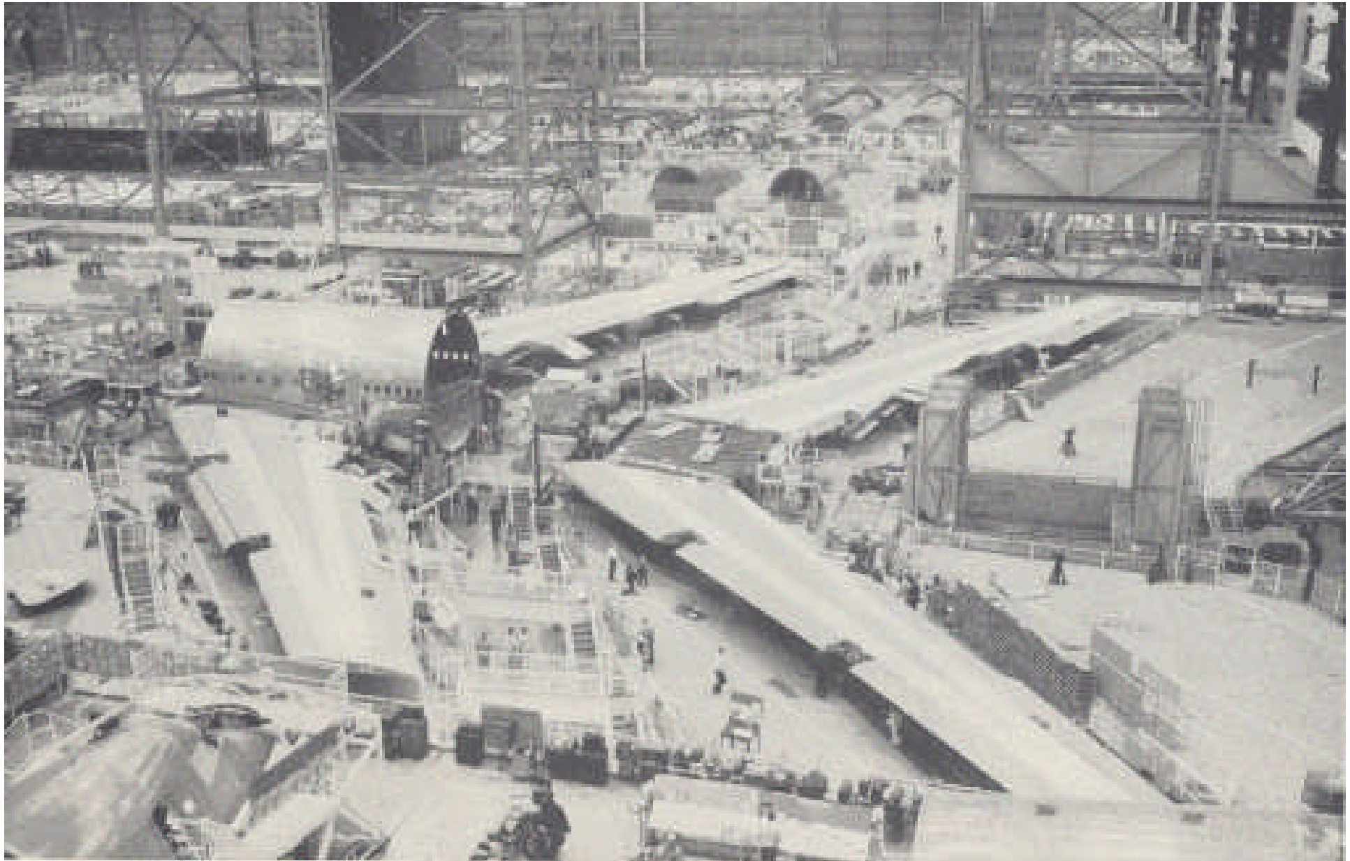
Above: caption: “Wing-body join station precedes joining of the three main fuselage sections at the next station. Station shown is in one of two final assembly bays in use. 446 A third bay is used for subassembly work.”
