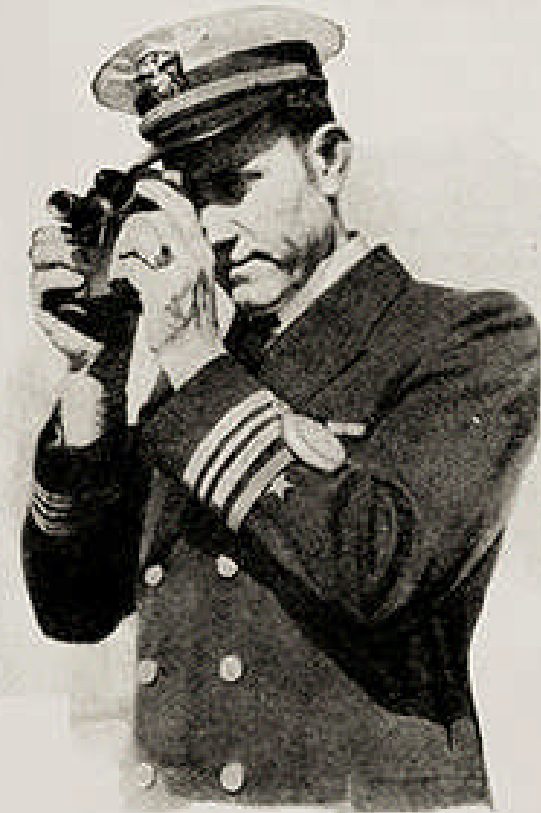
Lindbergh's tutor in the science of navigation, Lieutenant Commander Philip V. W. Weems, U.S.N., demonstrates the simplest method of taking bearings, using a sextant and the wrist watch seen on his left arm.
