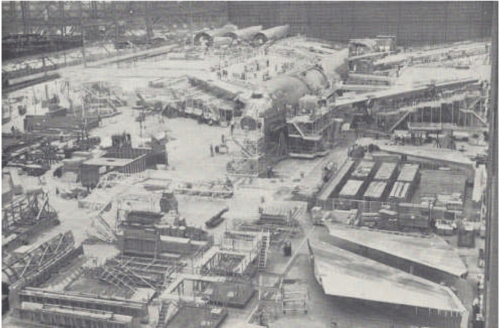
Above: caption: “Final body join position, where three major sections are fastened together, is located forward of the wing-stub join area. Landing gear and tail also are installed here.”
