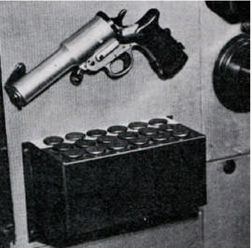
Above: caption: "Very pistol for emergency night signaling. The cartridge case beneath it contains red, green, and white flares."
