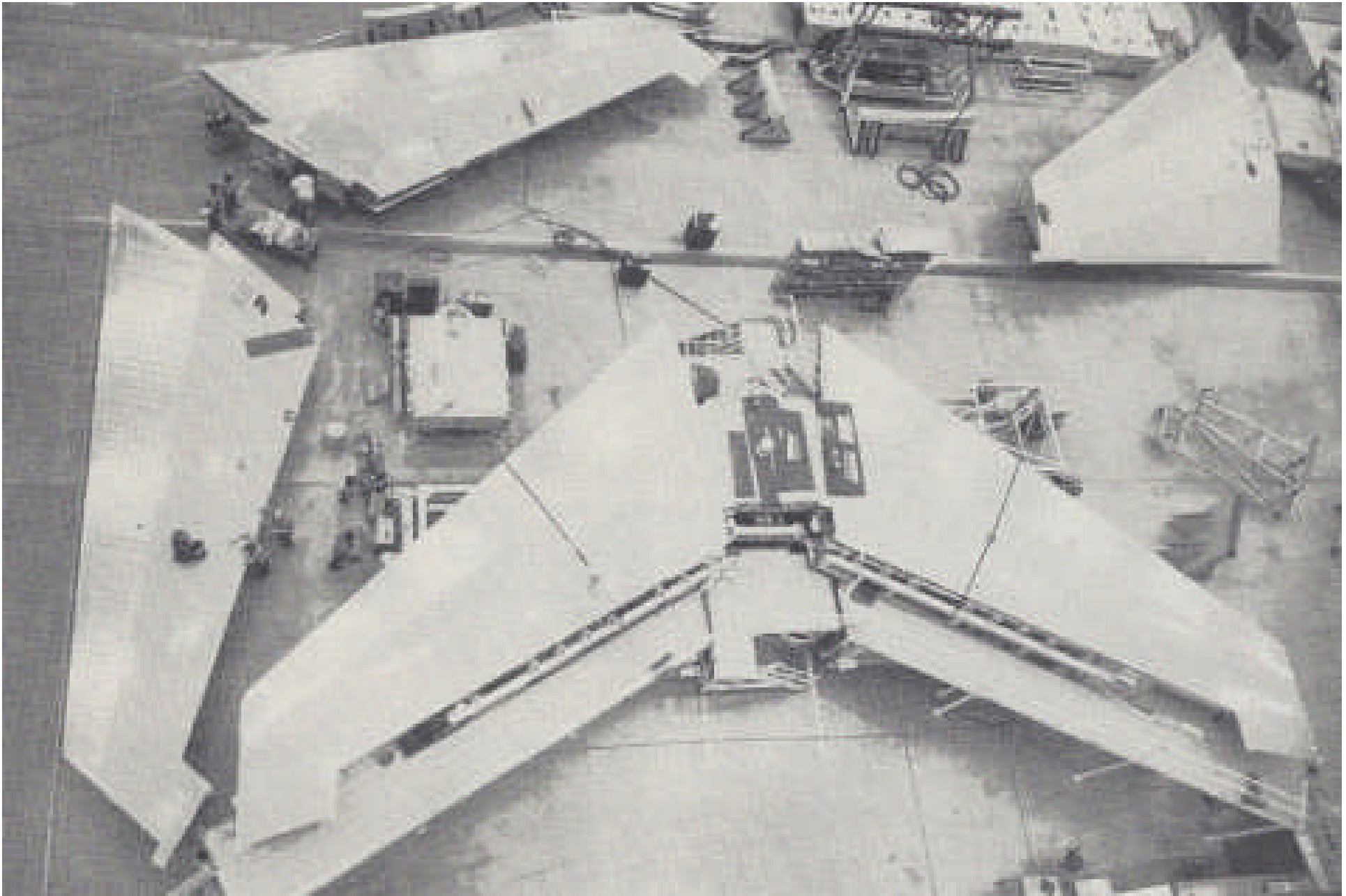
Above: caption: “Horizontal tail is built much the same as the main wing, with each stabilizer attached to a carry-through section to form a single unit. Elevators are installed after stabilizers are mounted to rear fuselage.
