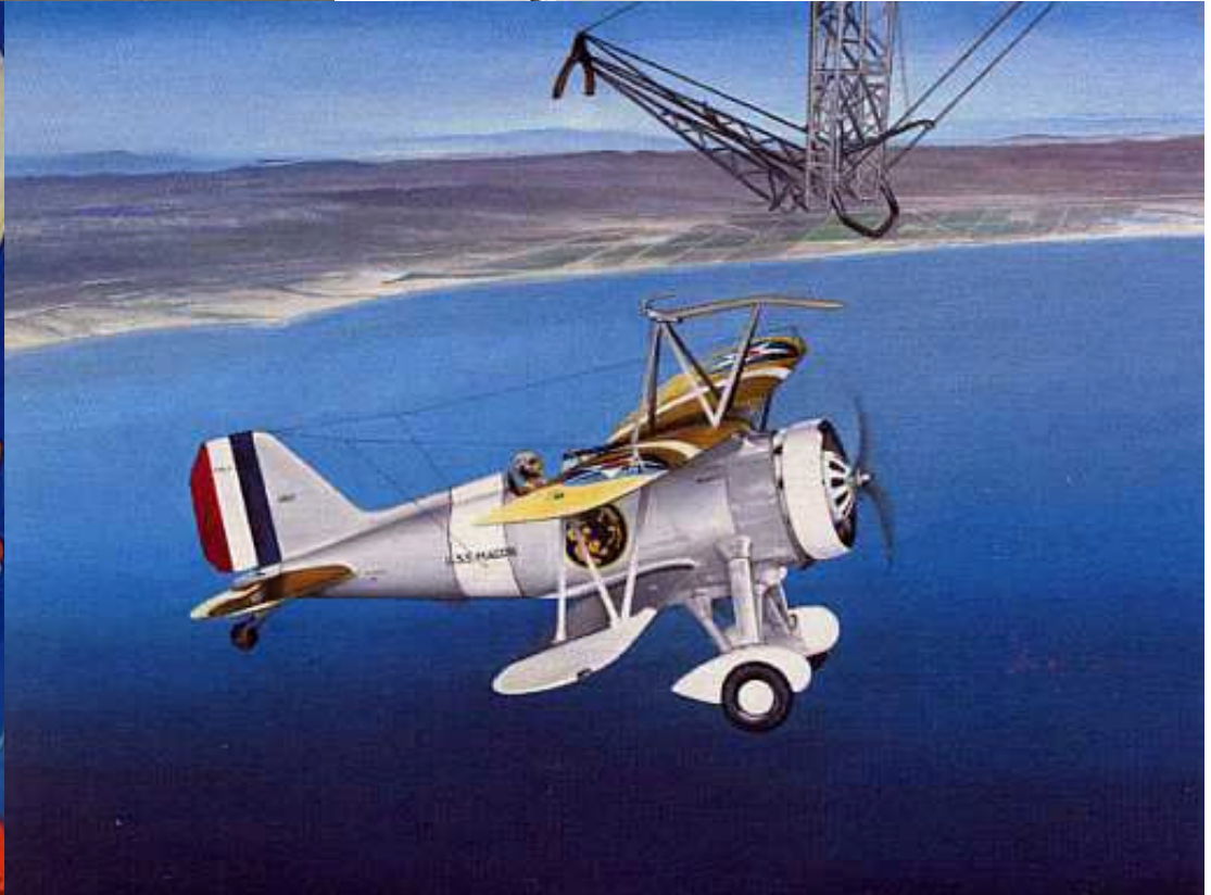
Above & Left: the use of LTA (Lighter-Than-Air) dirigible to launch and recover HTA (Heavier-Than-Air) fighter aircraft (ca. 1930s)
