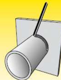
Pipe fixed horizontal axis, welding uphill: PH/5F
