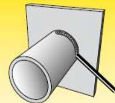
Pipe fixed horizontal axis, welding downhill: PJ/5F
