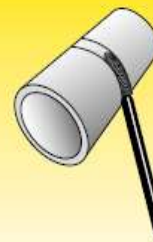
Pipe fixed horizontal axis, welding downhill: PJ/5G
