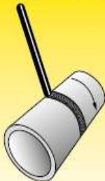
Pipe rotates horizontal axis Downhand: PA/1G
