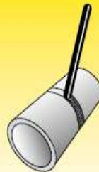
Pipe fixed horizontal axis, welding uphill: PH/5G
