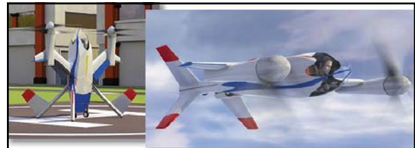
“...NASA is designing a one-person electric helicopter/small-aircraft hybrid for commuters...Known as a loner, the puffin is an awkward-looking bird with wings that seem too small for its rotund body. It's appropriate, then, that engineers at NASA adopted the moniker for their bizarre one-person aircraft that takes off from an upright position...” Popular Mechanics, January 2011 Above L&R: caption: “The Puffin is a conceptual design developed by NASA Langley. Designed to take-off and land vertically like a helicopter and fly like a plane, the craft has carbon composite construction and weighs less than 400 pounds, including the lithium phosphate batteries. The craft is shown in an artist's rendering parked in its vertical position (left) and in flight showing the pilot in the prone position (right).” 696
