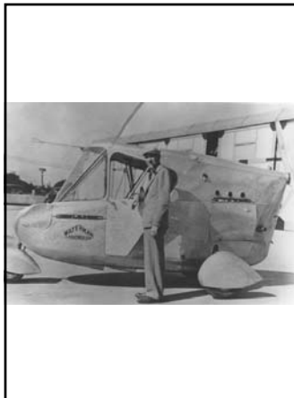
Left: caption: "Waldo Dean Waterman with his Arrowbile , 1937." Waterman was an accomplished aircraft designer who had worked for Curtiss Aircraft (by 1937, he had been working on flying cars for twenty years, including the famous 1917 Curtiss Autoplane ). The Arrowbile was only 20-feet long with a 38-foot wingspan. Its 100-hp Studebaker engine propelled it at 56 mph on the ground and 112 mph in the air. 407
