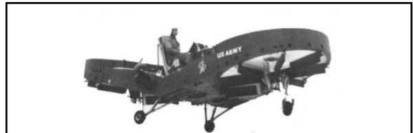
"...Both rotor-props will be shielded for safety and the Sky Car will hold a driver and three passengers. It will be able to fly down narrow streets or get above heavy traffic. It will also have powered wheels to drive it in and out of the garage or congested areas. According to Piasecki, the Sky Car will cost little more than a high-priced motor car of today..." Mechanix Illustrated , October 1958
