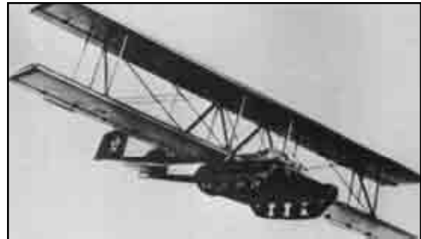
Above: the Antonov KT was developed in 1940 by a designer of weight-carrying gliders; Oleg Konstantinovich Antonov . The aim was to test the viability of supplying partisan forces behind enemy lines with light tanks. The unit was towed by a heavy bomber such as the Petyakov Pe-8 . A model T-60 light tank provided the fuselage of the unit (the unlocked tracks were the landing gear). Upon landing, the flying surfaces (i.e. wings, tail boom etc.) were to be detached and abandoned.
