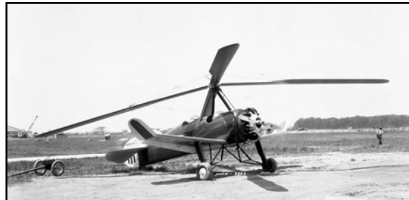
Above: caption: "The 1923 Pitcairn PCA-2." In many respects, the Autogyro is the true predecessor of flying cars. Harold Pitcairn's PCA-2 was the first rotary-wing aircraft to achieve type certification in the U.S. and was mass marketed. In one memorable promotional stunt in 1931, pilot Jim Ray famously landed and took-off from both the White House lawn and from a parking lot in front of the Capitol Building in Washington D.C.
