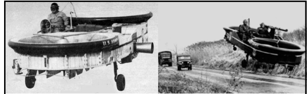
Above: the first of two Model 59 examples ordered by the Army made its initial free flight in October 1958 and was renamed "Airgeep" (left). The machine was subsequently given the designation "VZ-8P" (P=Piasecki). Shortly after being accepted by the Army, the VZ-8P was fitted with a single 315kW Turbomeca Artouste IIB turbine engine. Its first turbine-powered flight took place in June 1959. The craft was subsequently loaned to the U.S. Navy for evaluation (as Model 59N) and, upon its return to the Army, its Artouste IIB was replaced by a lighter and more powerful AiResearch 331-6 turbine. The second VZ-8P incorporated several significant design changes and was, accordingly, dubbed the "Model 59H Airgeep II" and the VZ-8P (B) by the Army. A subsequent five man model was fitted with an ejection seat for the pilot and gunner (right). Though the Airgeep was able to hover near the ground or fly thousands of feet in the air and it surpassed its competition in terms of performance, the Pentagon felt it wasn't suitable for the modern battlefield and the project was cancelled. 254
