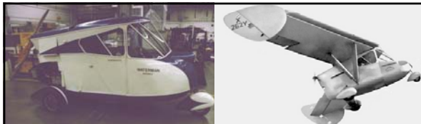
Begun in 1947, the Aerobile (span 38 ft; length 20 ft; height 8 ft 11 in; weight 1,710 lbs.) was fabricated from parts of Waterman's earlier designs. Completed ten years later, it was test flown in May of 1957. Its engine was mounted in the rear of the fuselage and power was transmitted to the pusher propeller and/or the two rear wheels (the propeller was not removed for ground operation). The tailless fuselage and quickly detachable wings allowed three-minute conversion from flying to road configuration. Ailerons and wing-tip rudders were interconnected (turns were made by turning the wheel, there were no rudder pedals). The three-wheel (tricycle) landing gear configuration allowed registration as a motorcycle in California. Top speed was about 70 mph on the ground and 120 mph in the air. It was noted that spins were nearly impossible and the Aerobile was very difficult to stall. One proposal was to sell the car and rent wings at local airports. Waterman based his Aerobile design on two previous efforts; Whatsit , a tailless plane of 1932 and Arrowbile , delivered to the Department of Commerce in 1935 as part of the "Safe Airplane" competition.
