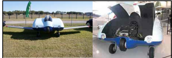
The Trautman RoadAir (left) was a "lifting body" design that also incorporated a channel wing. This channel, along with an 85-hp flat-four, air-cooled Continental O-190 engine and pusher propeller placed directly aft of the pilot, provided additional lift to the aircraft (the engine drove both the propeller and the rear single wheel). A sleek design, the RoadAir had wings stored in the lower portion of the fuselage. Small doors on each side were opened to access the wings which were pulled out and then locked in place. This arrangement provided a total wingspan of 25-feet. A fourth wheel was added in front (presumably for extra stability when driving). The V-type stabilizers were replaced by a more conventional pair of uprights, joined by a horizontal stabilizer. Pedals in the cockpit controlled not only the rudders when airborne, but also the pair of wheels under the passenger compartment when driving (the pilot gained access to the controls by lifting the front hood and climbing into the cockpit (right)).
