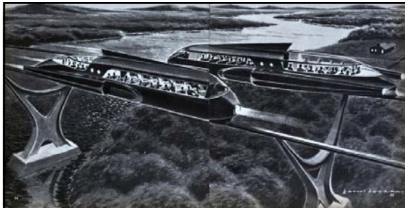
Above: caption: "Fantastic speeds of 200 to 500 mph are foreseen in the future for unwheeled vehicles using monorail system. Levapads would raise vehicle from rail, hold it away from rail sides." 231
