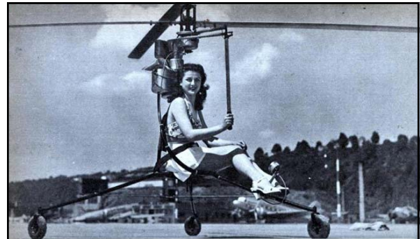
Above: caption: “Second version of the Hoppicopter design had a tripod landing gear with motor mounted behind the pilot’s head. It was better than the original ‘back strap’ model but weight distribution was unsatisfactory.”
