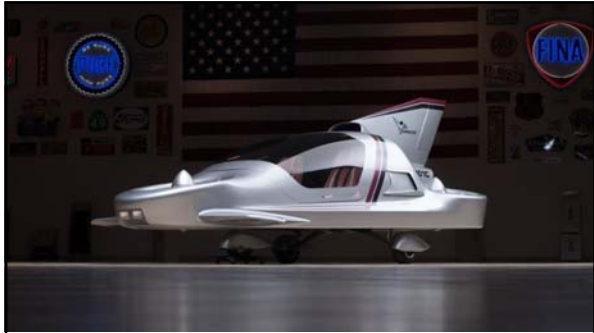
Above: caption: "The Sky Commuter (ca. 1990)." Developed by Boeing in the 1980s, for just $71,500 you could own the Sky Commuter concept car. Powered by a gas-turbine engine linked to helicopter-like driveshafts, the Sky Commuter was to be an alternative to the plane-strapped-to-car designs of the previous decades. Boeing spent $6 million developing the concept, but it never went into production. 19
