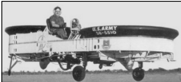
"...Piasecki's Flying Jeep is a radically different ducted-fan VTOL. Intended for military hedgehopping it has exciting possibilities as the forerunner of a family car that can fly. It consists largely of two huge horizontal ducted fans in tandem, with the pilot-driver seated between them. He uses vanes in the ducts to deflect the air flow for maneuvering..." Popular Science , September 1960
