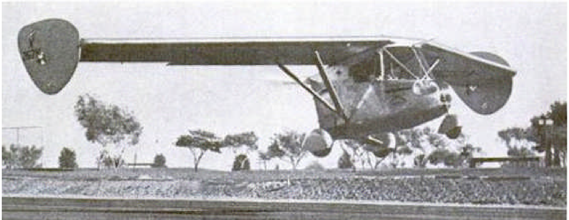
Above & Left: caption: “Detachable wings enable a vehicle of odd design to travel on the ground as well as in the air. Capable of attaining a speed of 110 mph while flying and 55 on the ground, the novel craft is powered by a standard six-cylinder automobile engine. Above, the auto-plane making a landing; Left, the auto-plane with wings detached for use on ground as a car”
