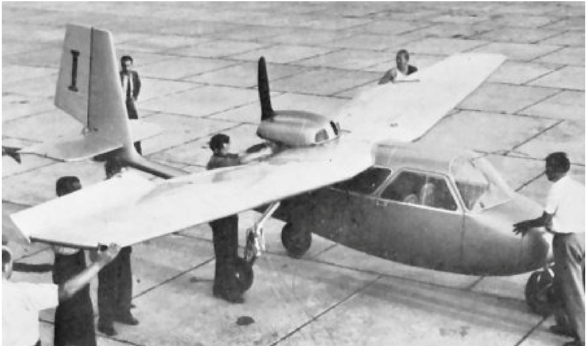
Above: caption: “Aerauto PL.5C Autoplane (1946-1953).” Luigi Pellarini, an aeronautical engineer, designed the Aerauto PL.5C , which was built by Carrozzeria Colli in Milan, Italy. Using the roadable aircraft with folding wings concept, Pellarini built the first roadable aircraft that relied on the same airplane engine for both flight and road travel.
