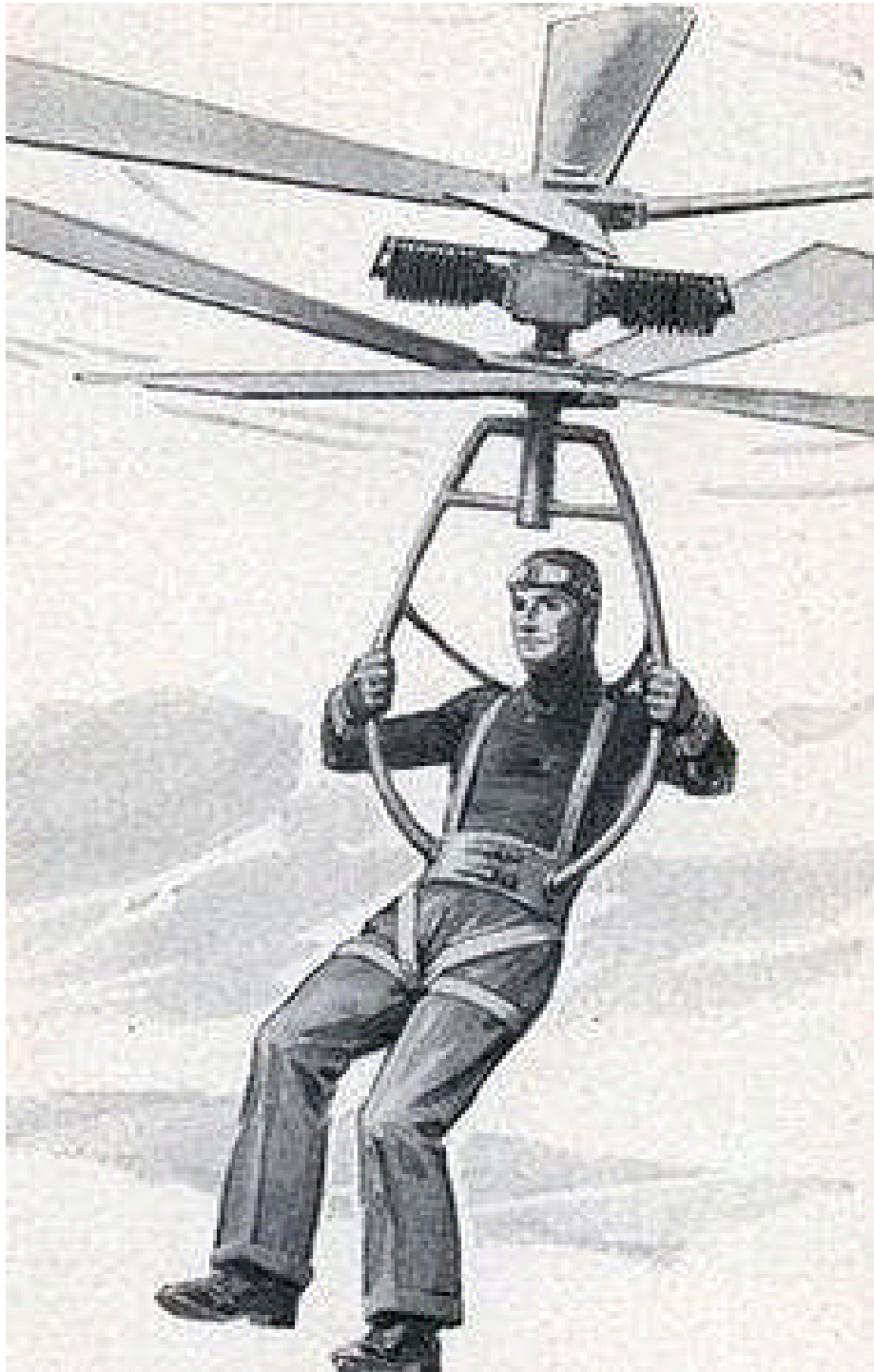
In 1940, George de Bothezat connected co-axial rotors to a body frame (left). Hiller later adapted it into a safer and more controllable “flying platform” (above).
