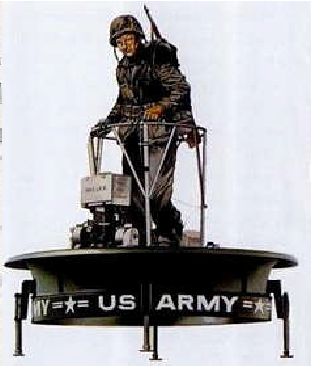
In 1940, George de Bothezat connected co-axial rotors to a body frame (left). Hiller later adapted it into a safer and more controllable “flying platform” (above).
