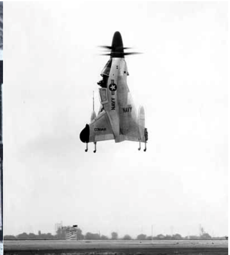
Above: caption: “The Convair XFY-1 ‘Pogo’ was a vertical takeoff and landing (VTOL) fighter that could operate from any deck, not just an aircraft carrier.”
