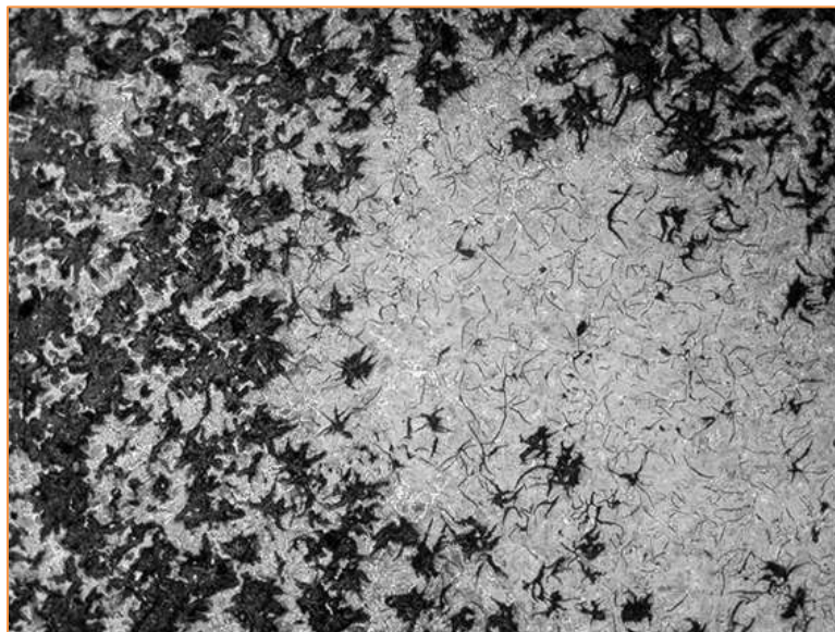
Graphitic Corrosion Attack in Gray Iron
