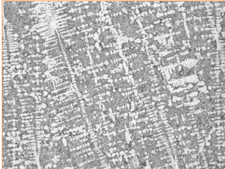
Gray Cast Iron Structure
