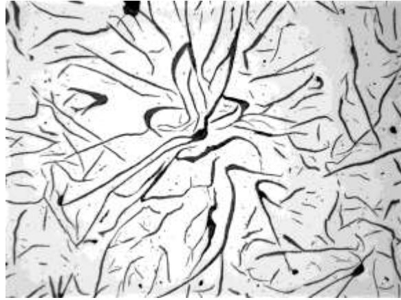
Inoculated gray iron structure
