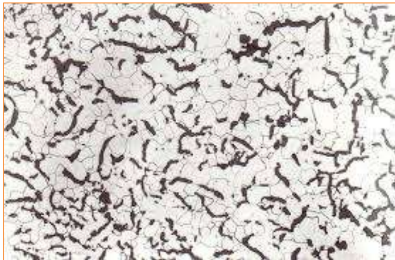
CG Iron Structure
