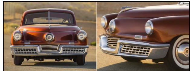
By May 1947, the front end of Clay No. 2 now incorporated Read Viemeister's steerhorn bumper as the backbone for the grillework. As of June 1947, the Tin Goose's front bumper and grille would remain virtually intact with the exception of a few missing slats in the centerpiece. The catwalk area above the bumper eliminated all chrome pieces, additional grilles, vents and/or turn indicators (as on both clay models). Tremulis did much of the lead solder filling and shaping on the deep drawn areas in the catwalk himself. The Tucker 48's front-end would add turn indicators to the areas just above the bumper, but remained, in essence, true to the spirit of the Tin Goose . 502
