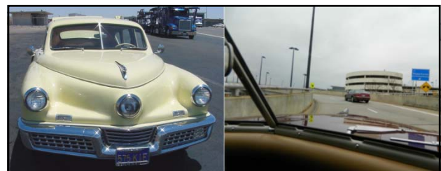
"...One of the most outstanding features was the safety windshield exclusive with Tucker. A laminated safety glass mounted in sponge rubber was fastened in such way, a hard blow from within would eject the glass in one piece. This, one of the greatest collision hazards - lacerations or a fractured skull from striking the windshield - was entirely eliminated. Also, the windows are made of armor-plate glass which disintegrates without cutting edges or slivers..."
