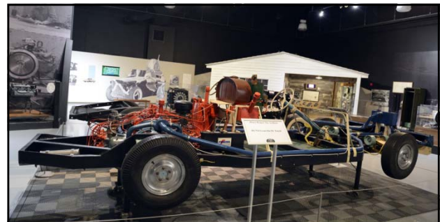
"...An exclusive with Tucker was a frame lower than the wheels. This was made possible by locating the engine in the rear, which also eliminated the conventional drive shaft. Creating protection and stability, this 'all-around' frame added to the ultimate safety of the the whole machine..." CAR CLASSICS , October 1972
