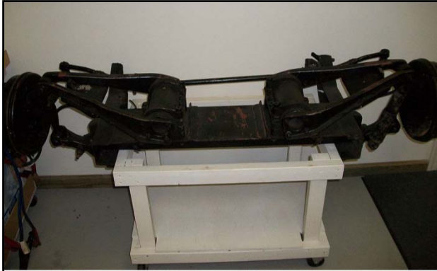
Above: caption: "Tucker Rubber Torsion Tube (version No. 2) - front suspension used on car Nos. 1026 on. This unit taken from car No. 1046 for V8 conversion." 193
