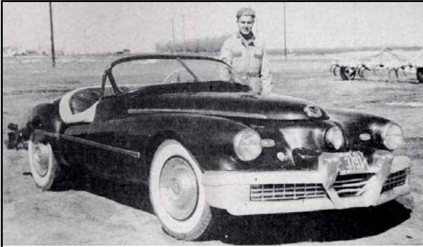
Above: George Esch built a fiberglass Tucker Convertible replica (completed in 1997). The car was based on a 1966 Chevrolet Corvair. He calls it the "Glass Goose." 1261
