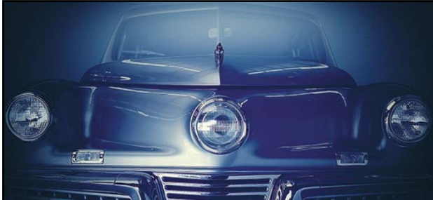
"...It has a third 'Cyclops Eye' headlight mounted in the center of the hood. This light is connected to the steering apparatus so that a beam of light turns and illuminates curves as the front wheels turn right or left..." Popular Mechanics , September 1947 RE: the most recognizable feature of the Tucker 48 was a directional third headlight; the "Cyclops Eye," that would activate at steering angles of greater than 10-degrees to light the car's path around corners. At the time, seventeen states had laws against cars having more than two headlights (Tucker fabricated a cover for the center light for use in these states). 139
