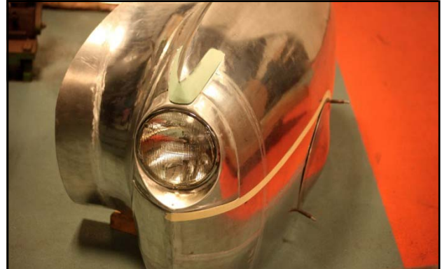
Above: caption: “Completed (and steerable) front fender pod” 1310
