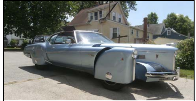
Above: this Tucker "replica" is attempting to reincarnate George Lawson's Tucker Torpedo design using a 1971 Buick Riviera. According to the seller on ebay, his uncle built the car as a labor of love and, supposedly, used actual plans from Tucker as his inspiration. Some of the replica's modifications include front fenders that turn with the wheels and a fin running down the back. All three headlights work, but the one in the middle is only for high beam. The hinged sections on the roof are meant to open to make getting in and/or out easy-on-the-skull. According to the eBay auction, the car was not in running condition and was in need of some restoration. A reserve of $7,300 was set for the auction. 1262
