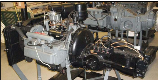
It was also becoming clear that many of the breakthrough designs Tucker called for and featured in their early advertisements could not be implemented (at least not at the car's projected selling price of $2,450). The Ben Parsons designed flat-six (589 cu. in.) engine was proving troublesome, so the decision was made to fit production models with a Franklin six-cylinder engine. As well, an Alex Tremulis design for a fastback sedan body style (with conventional seating for six) was chosen for the final design. 125 Above: caption: "Franklin O-335 engine and Tucker Y-1 transmission"
