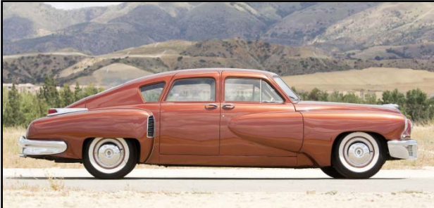
"...It is by far the most comfortable automobile I have had an opportunity to ride in. The head room is remarkable. This is due to another exclusive Tucker feature, roof top doors. All four doors are curved at the top; opening well into the roof itself giving ample room for entering or exiting the car. There is no need for a passenger to jack-knife his body, or bend and twist like an eel to enter the car..." 667 CAR CLASSICS, October 1972
