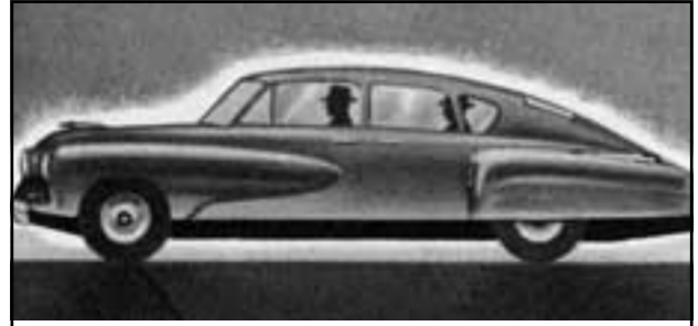
"...In spite of this unbelievable roominess inside the car, it is only five feet from road to roof. This low profile is accomplished by a step down floor only nine inches above the pavement, which still affords greater road clearance than comparable 1972 cars, 24 years since the last tucker rolled off the assembly line..." 668 CAR CLASSICS, October 1972
