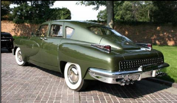
For the roll-over scene, a total of three cars were used; a fiberglass pre-crash version with no body damage (above), a modified Studebaker (which was actually driven and rolled by a stunt driver) and a post-crash version (which replicated the damage of car No. 1027). The fiberglass body was fitted onto a Ford LTD chassis. 1255
