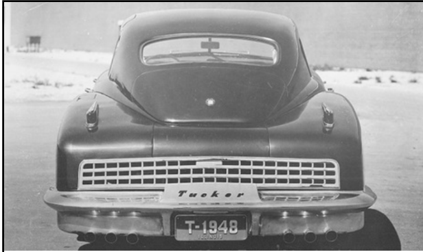
Above: caption: "June 18, 1947: The rear of the Tin Goose." The grille was modified for three rows and the individual exhausts were moved from within the bumper to half-underneath the bumper. The Tucker nameplate was added to the riser on the bumper. 481
