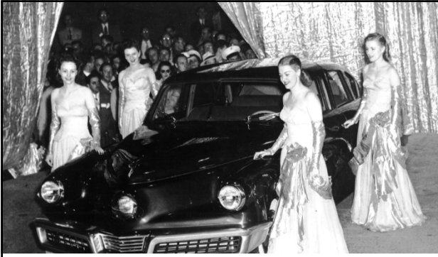
Above: the Tucker 48 premiered in the Tucker plant before the press, dealers, distributors and brokers. Tucker later discarded many of the prototype's features such as the 24-volt electrical system starter to turn over the massive 589 cubic-inch engine (for the premiere, workers substituted two 12-volt truck batteries weighing over 150 pounds that caused the Tucker's suspension arms to snap). Speeches dragged on as workers behind the curtain worked feverishly to get the prototype ready. Finally, before the large crowd, the curtains parted and the Tucker automobile rolled down the ramp from the stage to its viewing area where it remained for the rest of the evening. 121
