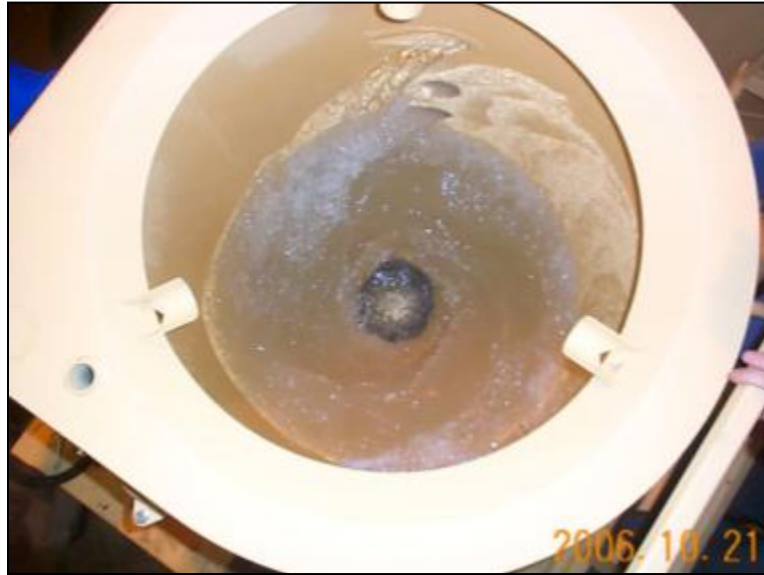
Figure 10-5. Vortex inside a high-shear mixer.
