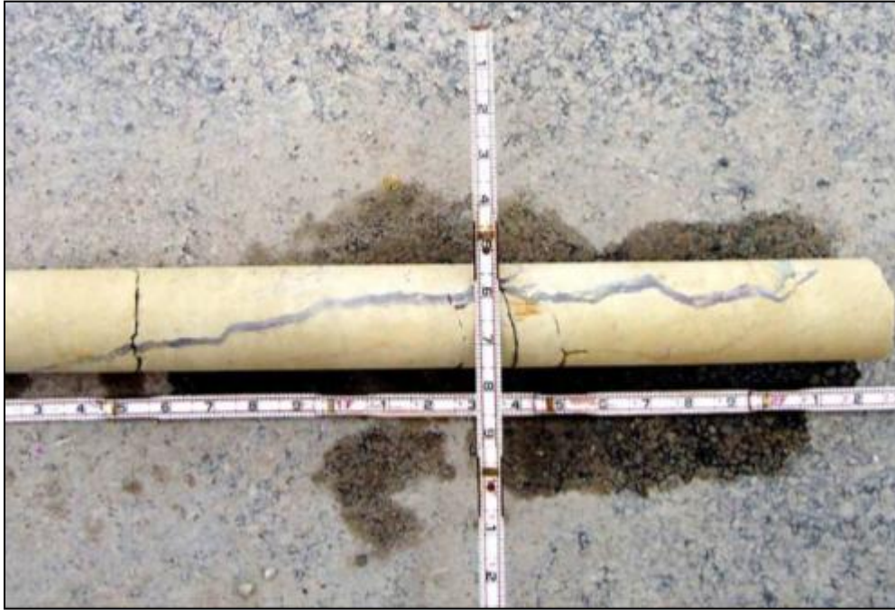
Figure 17-41. Large, clean fracture in limestone completely filled with grout.
