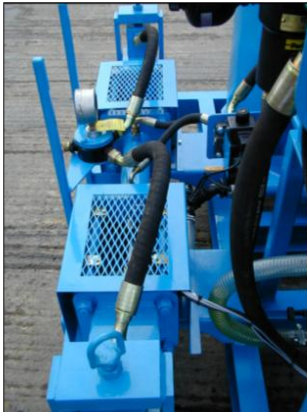
Figure 10-11. Piston pump with a reciprocating power source.
