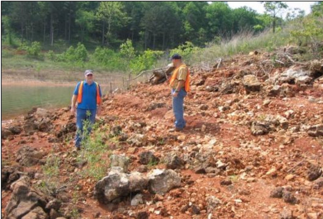
Figure 17-26. Clearwater Dam epikarst exposure (Little Rock District).
