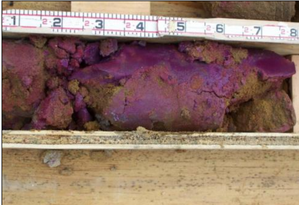
Figure 17-42. Soil sample from a sleeve-port grouted zone, with grout presence indicated by phenolphthalein and recovered grout lenses.
