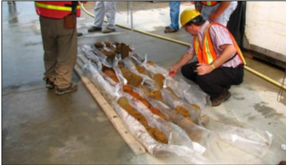
Figure 17-43. Overburden sampling program with a sonic drill at Wolf Creek Dam (Nashville District).
