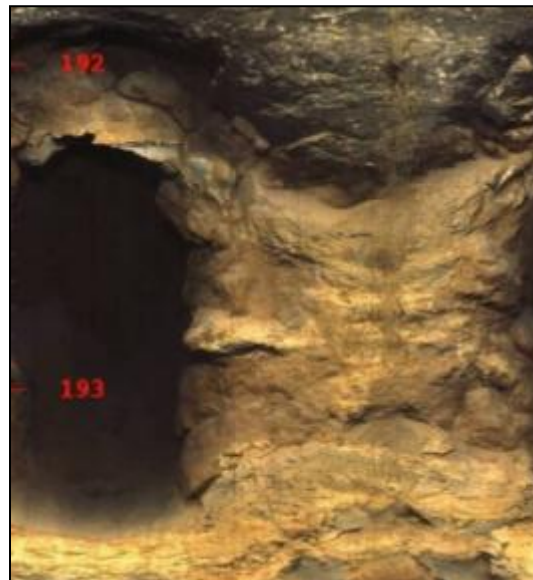
Figure 17-38. Clean 1-ft feature at Wolf Creek Dam, Leipers formation. The vertical scales are feet.
