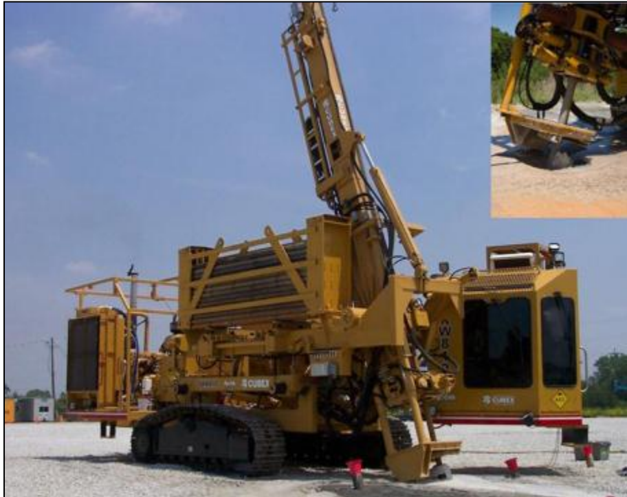
Figure 9-10. Water-powered down-hole hammer in action at McCook Reservoir. A large drill was used as depths exceeded 400 ft on this project.
