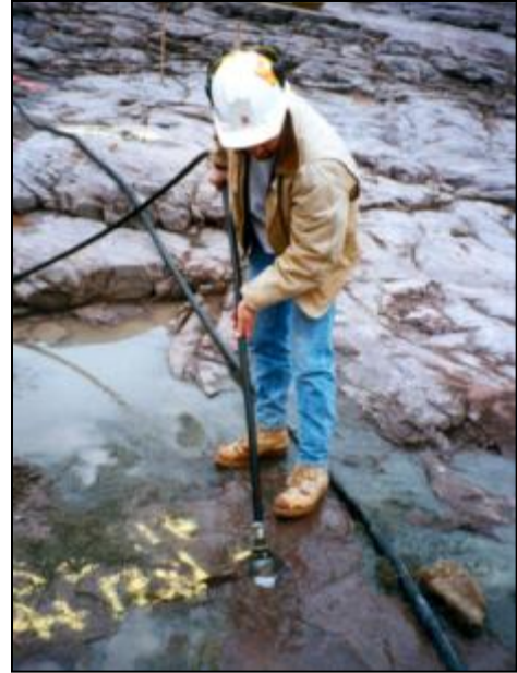
Figure 9-11. Lightweight washout bit and hose for manual applications.
