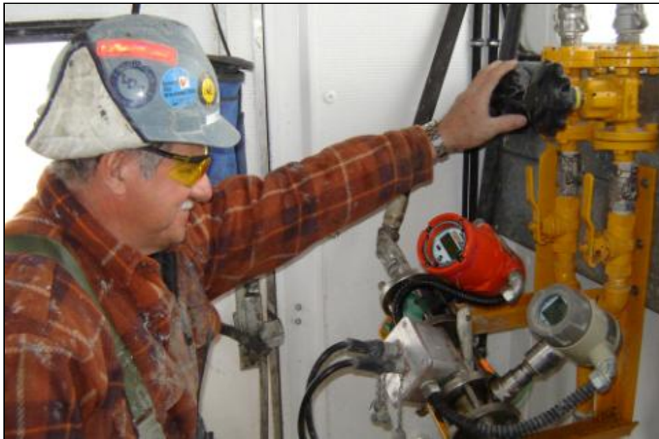
Figure 10-13. Header operator using a diaphragm valve on a return line to control injection pressure.
