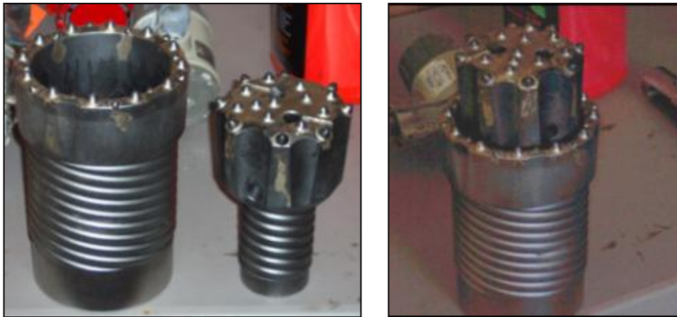
Figure 8-7. Example duplex casing shoe and drill bit.
