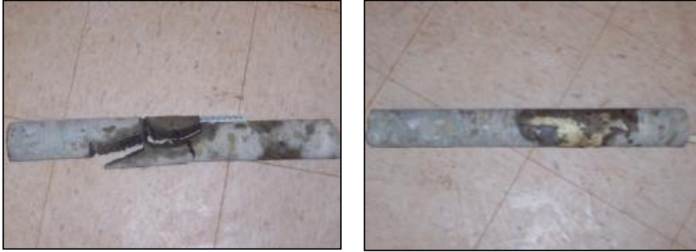
Figure 7-9. Concrete cores before and after grouting with urethane grout.
