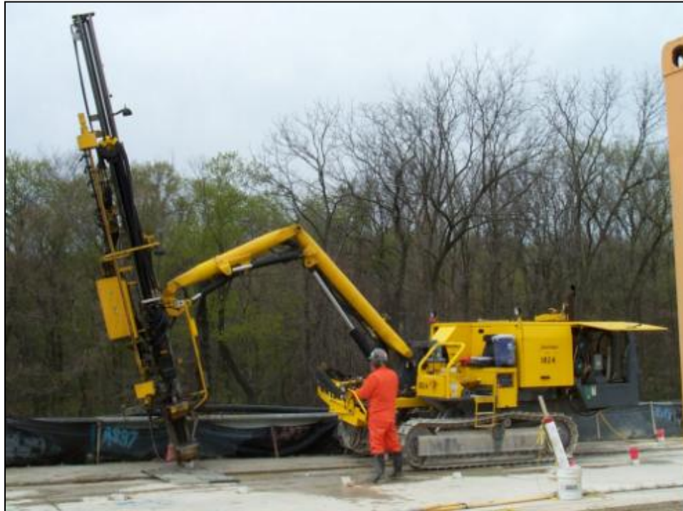
Figure 9-7. Self-contained, track-mounted, top-hole percussion drill with a rod handler.
