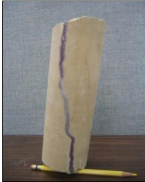
Figure 7-10. HMG-filled fracture. The grout is indicated in purple by phenolphthalein.
