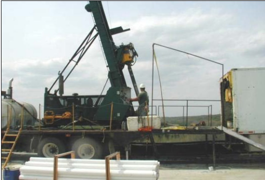
Figure 8-4. Sonic drill equipped with mast braced to permit angle drilling.
