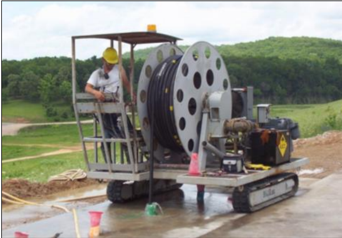
Figure 13-32. Wash water and cuttings being directed to an environmental control system.
