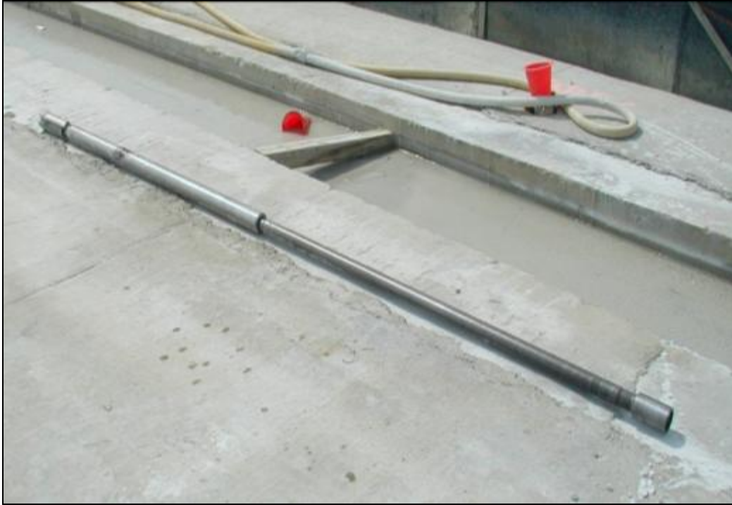
Figure 9-5. Top-hole percussion drill tooling. Bit is shown at top left followed by larger-diameter starter rod, followed by traditional drill rod.
