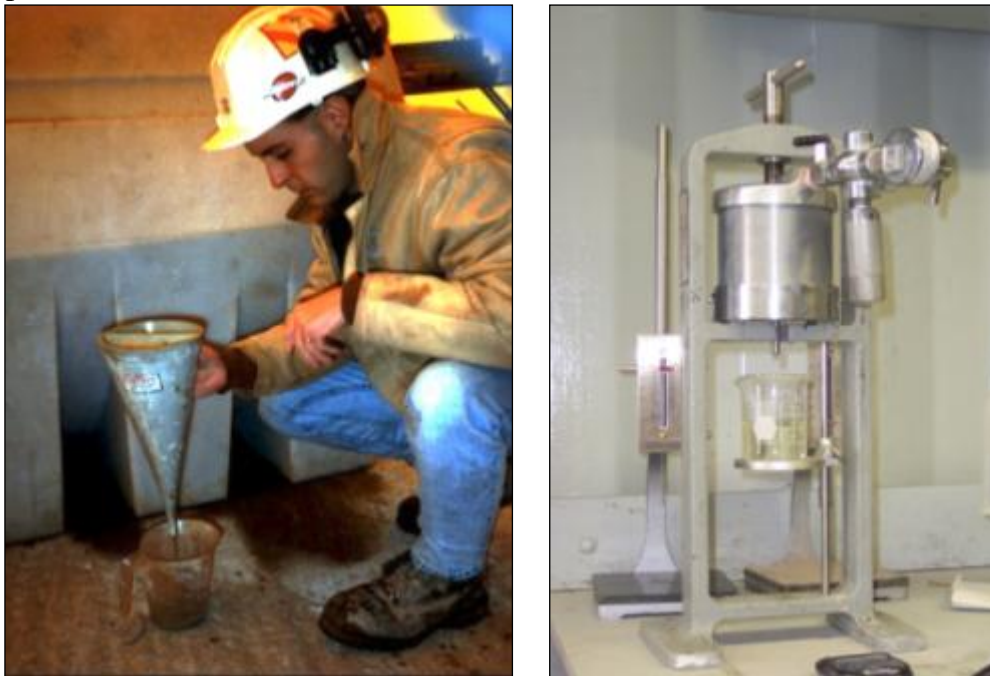
Figure 7-15. Testing for apparent viscosity and pressure filtration.
