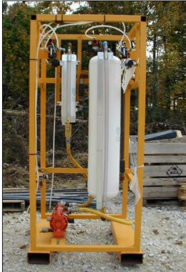
Figure 10-8. Pneumatic additive dispensers.
