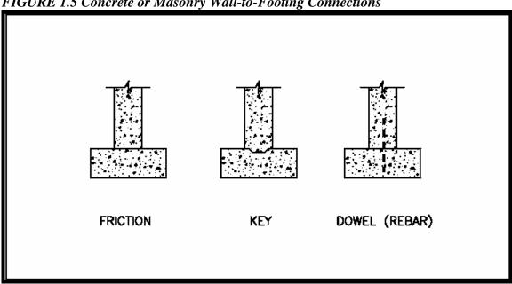
FIGURE 1.5 Concrete or Masonry Wall-to-Footing Connections
