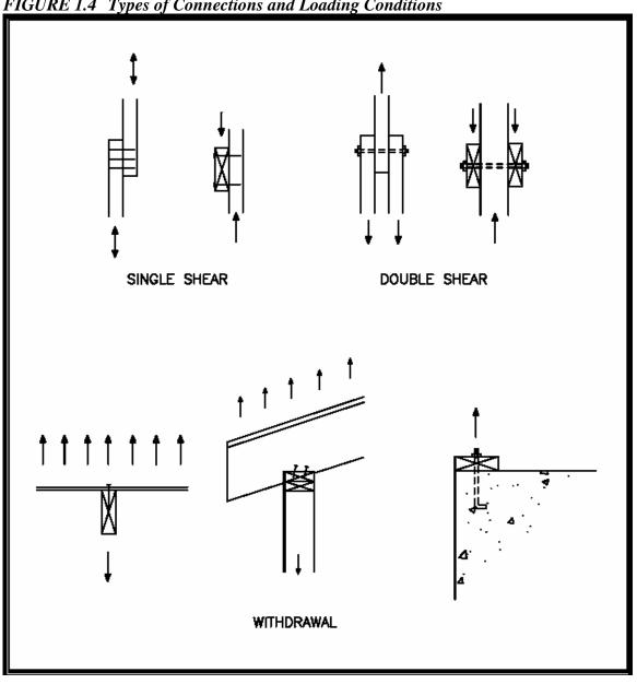
FIGURE 1.4 Types of Connections and Loading Conditions
