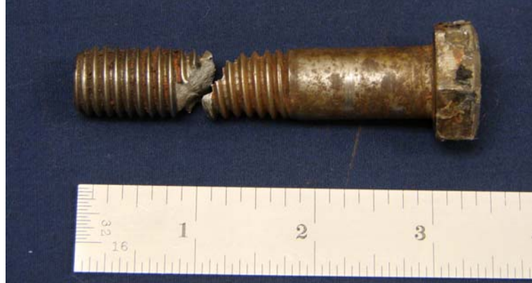
Figure 1. Photograph of a bolt after tensile testing, failure occurred in a ductile manner in the threaded section away from the head to shank junction area.
