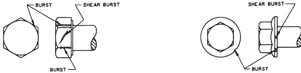
Typical Bursts and Shear Bursts
