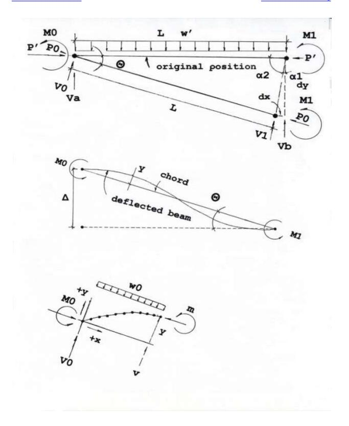
The third diagram shows a free body diagram of an initial portion of the beam. This results in the following equation,
