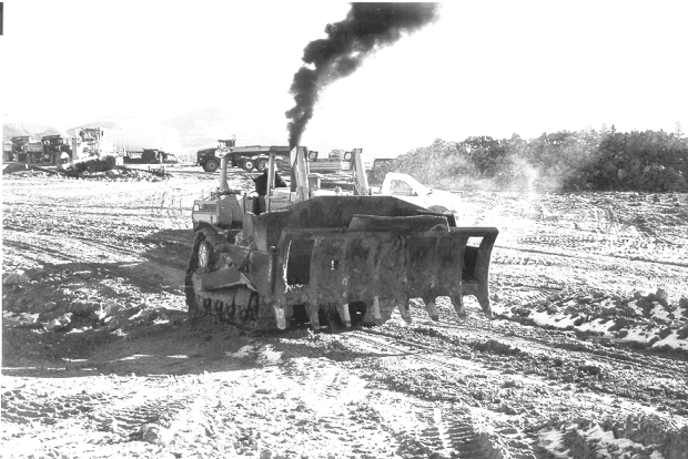
Figure 18-7.—Rock rake. A dozer-mounted rock rake separates the larger fragments from the smaller material.
