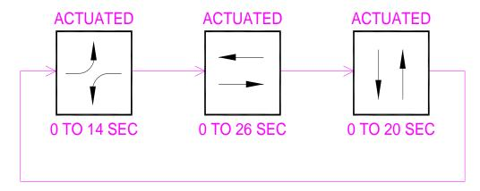
The cycle length will vary from cycle to cycle with a maximum cycle length for this example of 60 seconds. Fully-actuated controllers offer the most sophisticated timing features and capabilities so the remaining discussion centers on these types of controllers.
