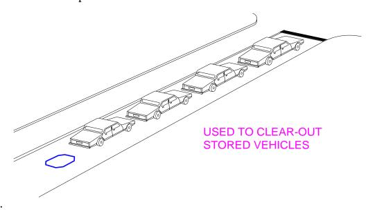
When the detection area is located <u>at</u> the stop line, the purpose of the initial interval is to ensure that a reasonable minimum green time is displayed, not a too-short green time that might violate driver expectation or a too-long green time that is wasteful.
