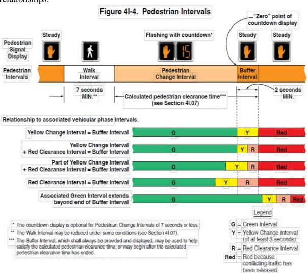
Countdown pedestrian signals, which are required by the MUTCD when the pedestrian change interval is longer than 7 seconds, display the number of seconds remaining until the termination of the pedestrian change interval.
