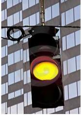
Based on this formula, the length of the yellow interval increases with increasing approach speed. The formula also produces longer yellow intervals for approaches located on downgrades and shorter yellow intervals for approaches located on upgrades.
