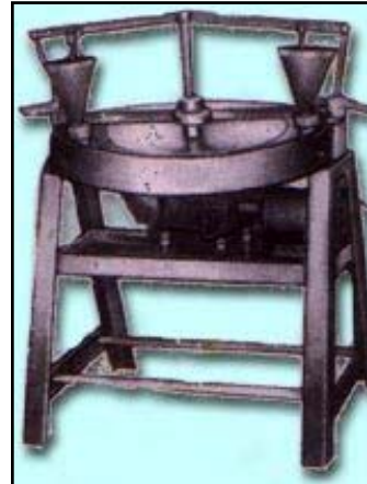
Left caption: "Dorry Abrasion Testing Machine"
