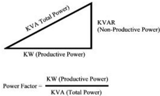
The cosine of the phase angle  $\phi$  between the KVA and the KW components represents the power factor of the load. KVAR represents the non-productive reactive power and  $\phi$  is lagging phase angle.
