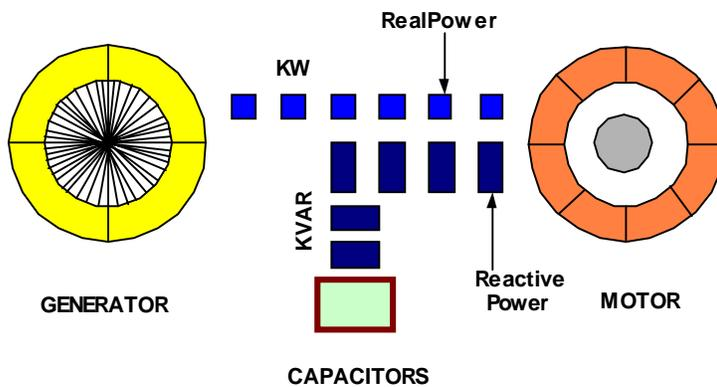
In the illustration above, addition of the capacitor has improved line power factor and subtracted the non-working current from the lines. Rather than transfer energy back and forth between load and generator, the reactive energy to supply the magnetizing current is now stored in a capacitor at the load, thus reducing the distribution requirements for excessive current. This reactive current supplied by the capacitor rather than the utility.
