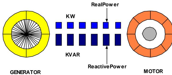
The figure below shows the results of installing a capacitor near the same motor to supply the magnetizing current required to operate it. The total current requirement has been reduced to the value of the useful current only, thus either reducing power cost or permitting the use of more electrical equipment on the same circuit.
