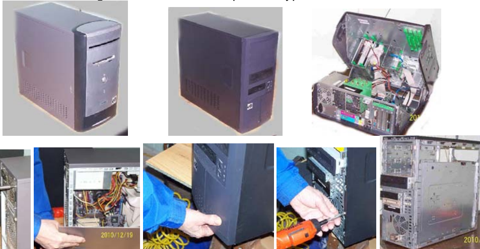
Remove rear screws left side cover pull up to remove front Remove front screws Front & Rt side mATX Computer----- ATX Computer-----
