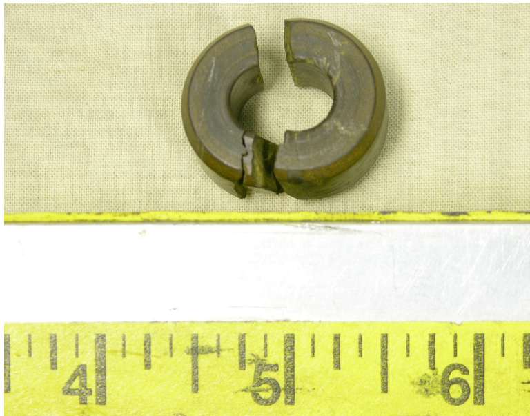
Photograph showing fractured roller
