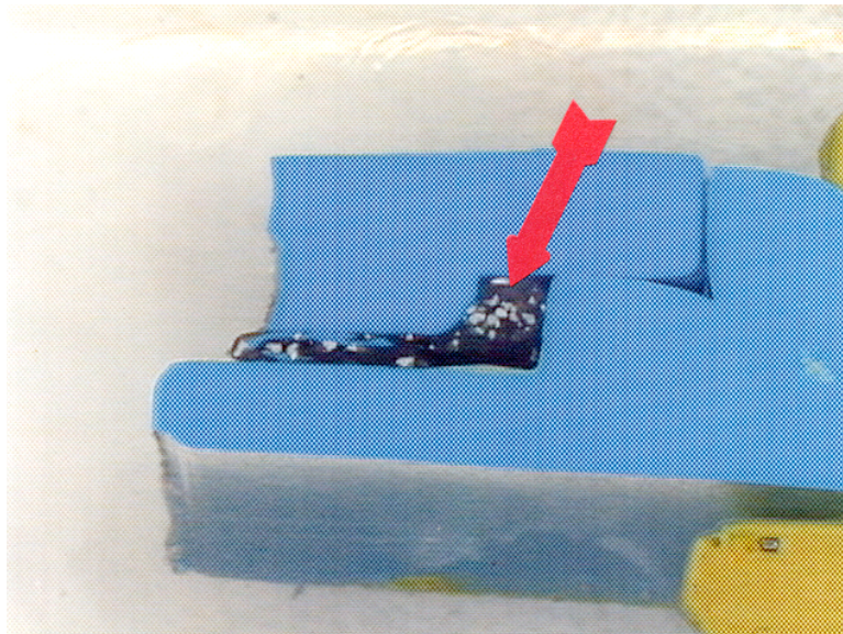
Cross sectional view showing the weld joint made using ferromagnetic particles
