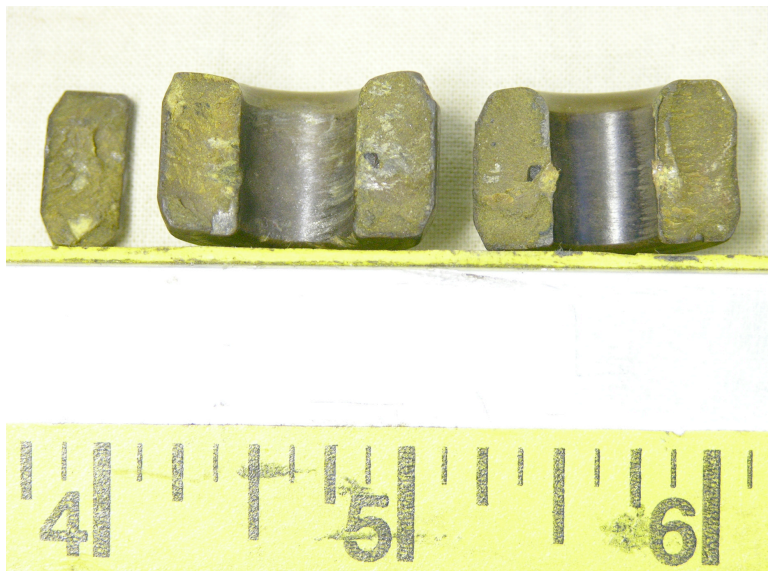
Photograph showing the fracture surfaces of the roller
