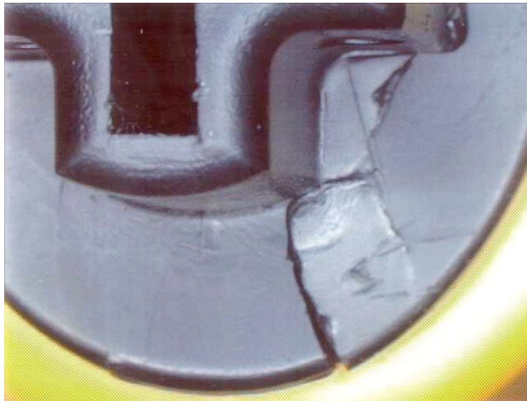
Close-up view of cracked insert
