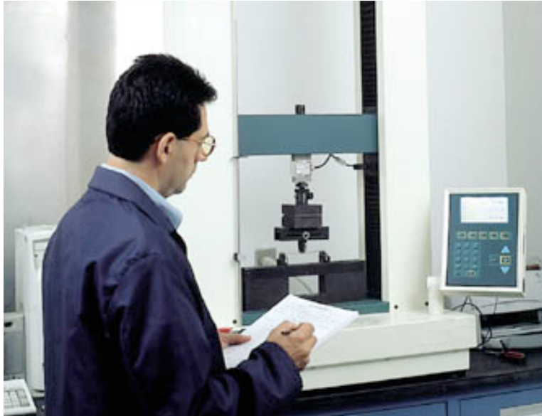
Photograph of a universal test machine showing the flexural strength test set-up
