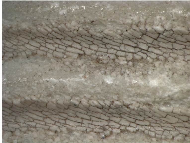
Photograph showing an oxidized/degraded surface due to natural weathering
