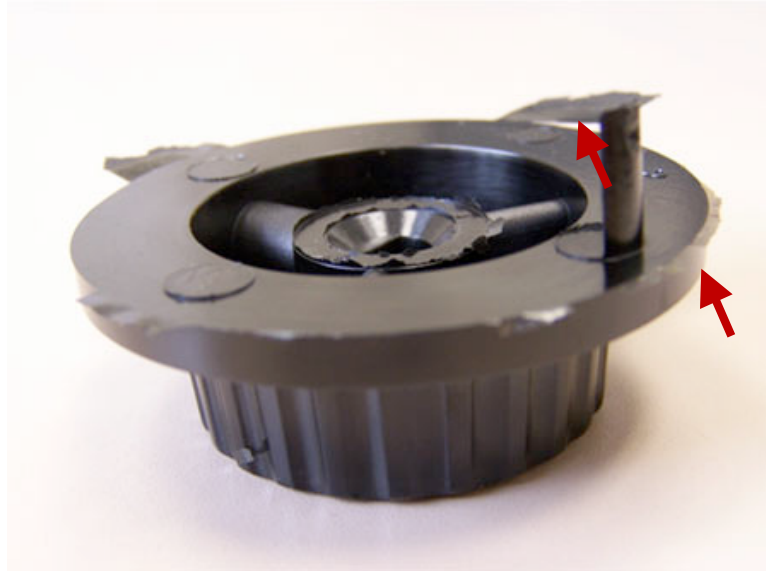
Photograph of a part exhibiting flash
