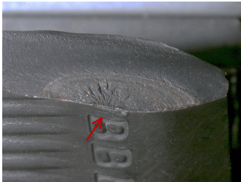
Fracture surface showing fatigue initiating at a stress concentration created by the indented lettering
