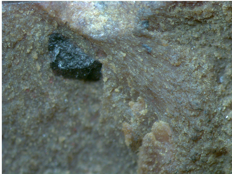
Higher magnification view of inclusion and origin area
