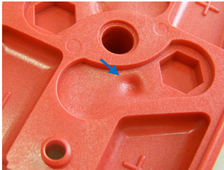
Photograph showing a sink mark
