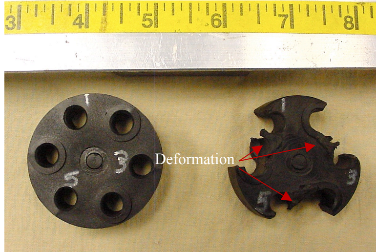
Photograph showing the failed and unused disks
