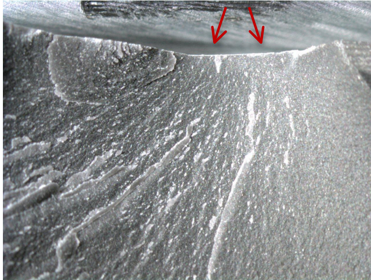
Fracture surface with chevrons pointing back to the origin
