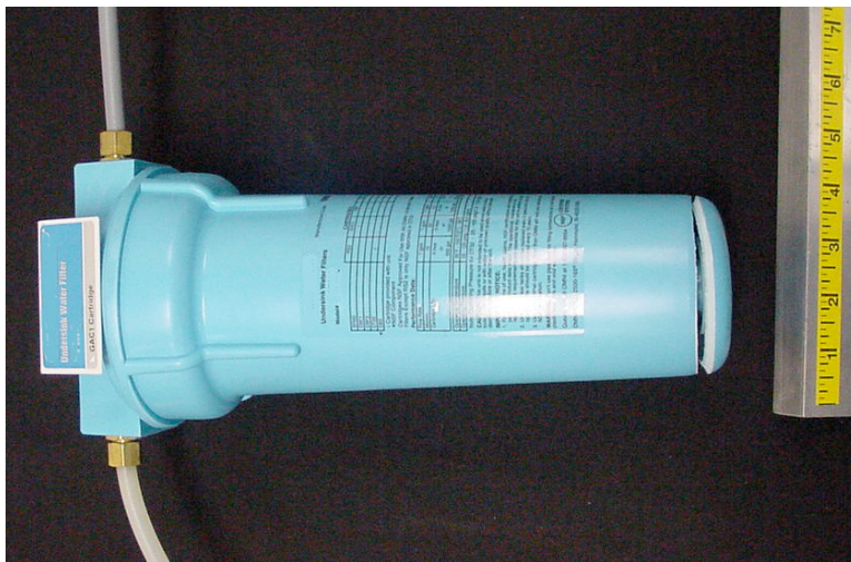
Photograph showing overall view of the cracked filter housing
