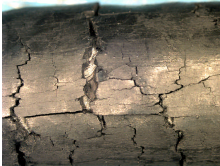
Environmental cracking was observed on the fuel hoses
