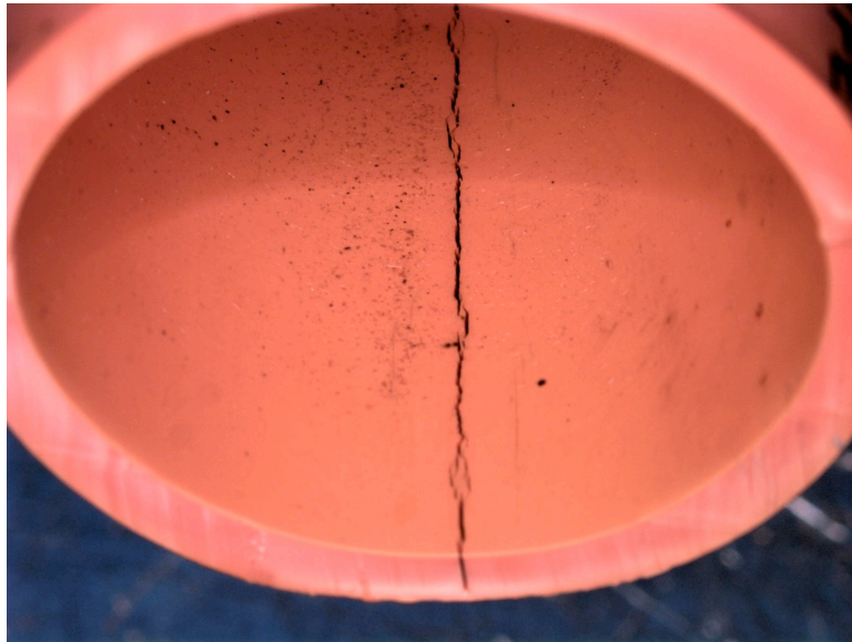
Close-up view of one of the longitudinal cracks in the failed section
