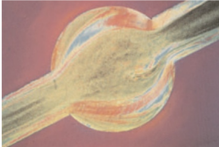
Inhomogeneous melt (brittle part)
