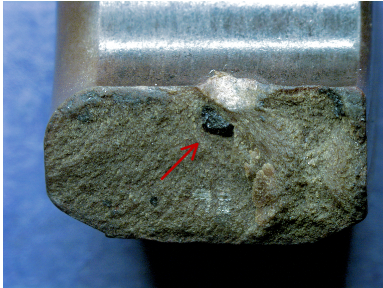
Macrograph showing the inclusion on the fracture surface (arrow)
