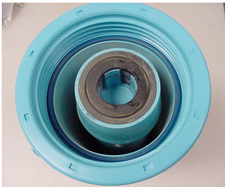
Photograph showing the cartridge and the housing interior after removing the cap
