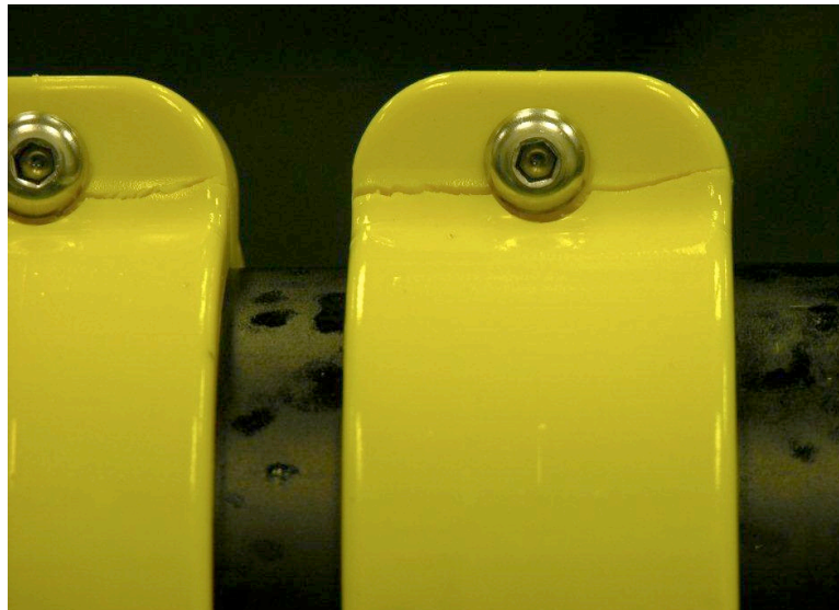
Photograph showing cracking that developed around the high stress areas of a clamp upon exposure to a cracking agent
