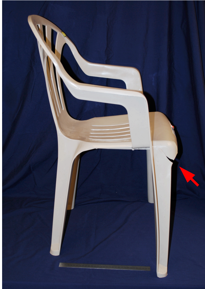
Photograph showing the chair, with arrow pointing to the fracture location
