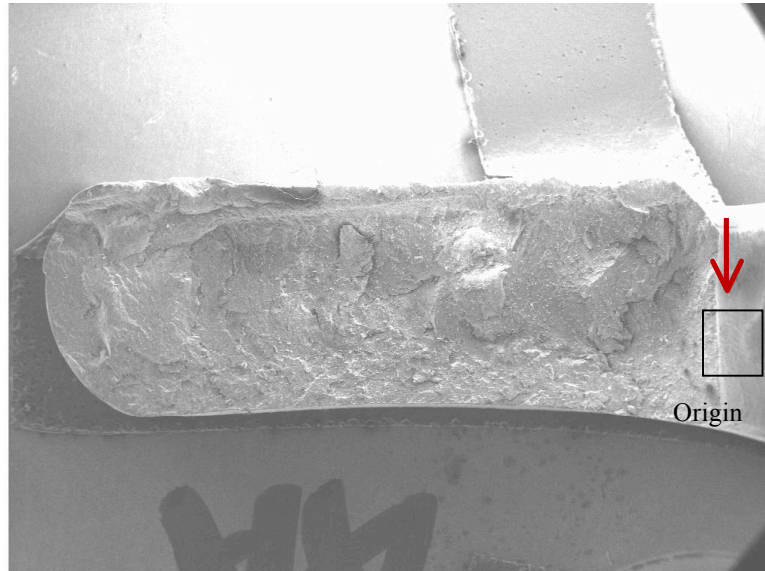
Fracture surface of one of the cracks, origin on right
