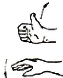
Lower load and raise boom
