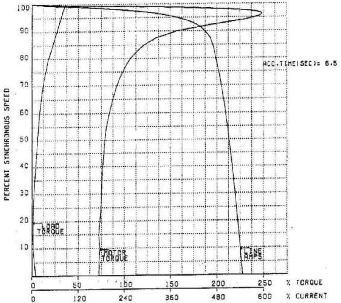
The necessary values can be determined from the motor torque versus speed curve. Note that the torque versus speed curve for the compressor is included. The driven equipment's manufacturer typically provides the torque versus speed curve for the load. The starting condition for the driven load should be checked for initial conditions and if possible the required torque should be minimized to reduce the starting condition on the motor.
