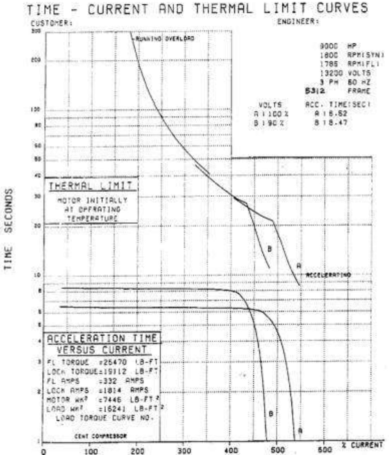
The time – current curve also provides the thermal limits for the motor during acceleration initially at operating temperature. The motor over current protection can now be selected to operate between the acceleration curve and the thermal limits to properly protect the motor during starting
