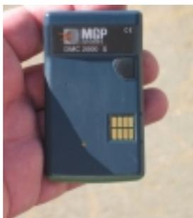
Most of the industry has migrated to the use of Personal Alarming Dosimetry or PADs. The reason is these devices have information programmed into them about the dose rates and maximum exposure you are allowed on a particular job. If the PAD detects you are in a dose field higher than allowed it will alarm. Also, if you exceed your dose limit the device will alarm (actual
