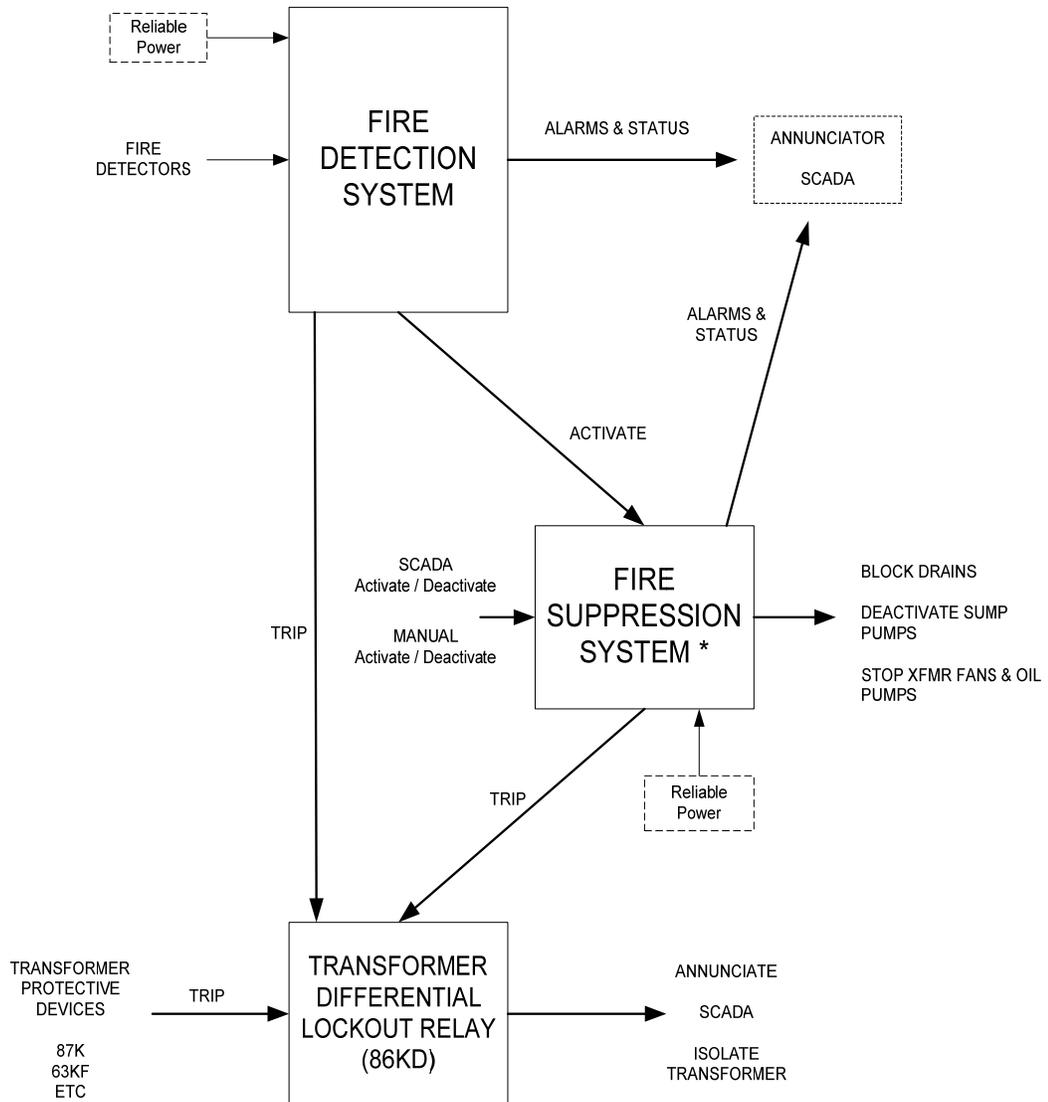
\* Includes electrical and mechanical equipment to discharge fire suppression water. Deluge type should cycle or use high level detection to limit water volume and overflow risk.
