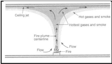
>>The field of fire science is now sufficiently mature that details of fire mechanics under a wide range of environments and influences can be accurately predicted. This sketch is the most simple representation. It is good for conceptual purposes, but lacks the detail available for analysis of real fires under real conditions.
