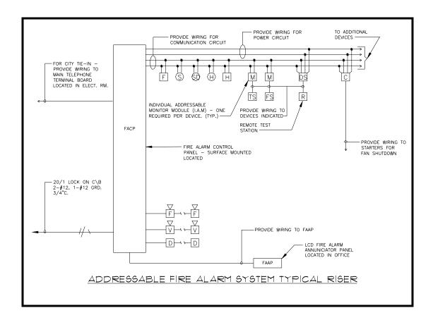
Note that this designer used different, though recognizable, symbols for the fire alarm devices. A characteristic of this example is the explicit indication of power wiring for the sensing devices. Wiring of the notification devices and interface is not similarly detailed. There have been no requests for information from confusion arising from this riser diagram.
