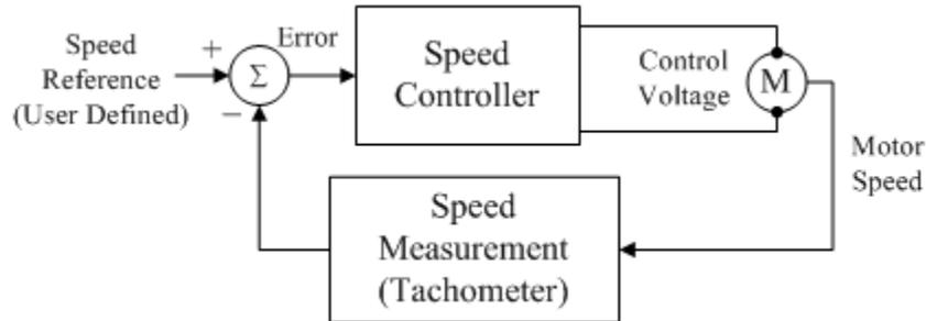
The speed controller contains two components: speed control and a digital-to-analog converter. The speed control component compares the desired speed with the measured speed and generates a digital value proportional to the DC value to be applied to the motor. The digital-to-analog converter is implemented using a signal generator and a low pass filter to smooth out the signal.
