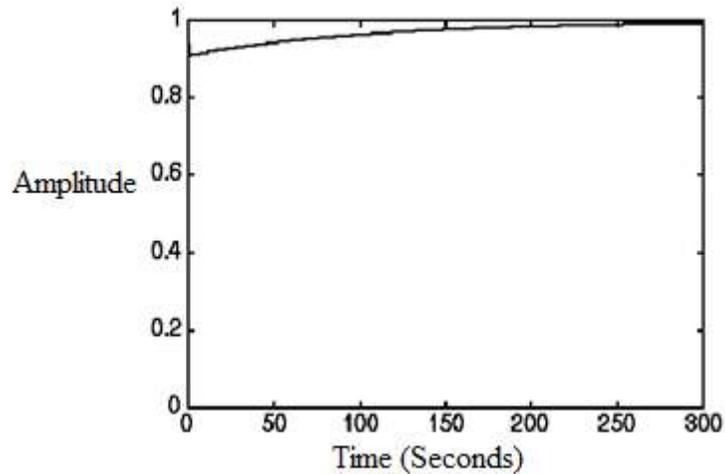
However, now the settling time is too long. So we increase  $K_i$  to 200 to reduce the settling time. After that, the step response curve looks like the following:
