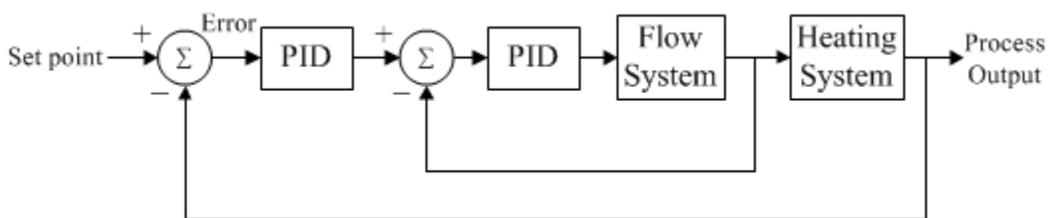
Cascade control is especially advantageous when the main disturbance is in the inner loop. This is because with the cascade configuration, the correction of the inner disturbance occurs as soon as the secondary sensor detects the upset. There are three main advantages gained by the use of cascade control:
