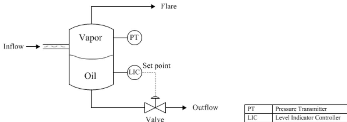
In this example, oil is flowing into the tank in a non-constant rate. The oil level in the tank is the process variable, which is measured, and this information is fed back to the controller. An operator enters a set point for a desired level. The controller compares the current level with the set point and generates a value that is
