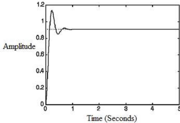
From the figure above, we see that both the steady state error and overshoot are too large. Since adding an integral term will eliminate the steady state error and a derivative term will reduce the overshoot, we try a PID controller with small  $K_i = 1$  and  $K_d = 1$ . After that, the step response curve looks like this:
