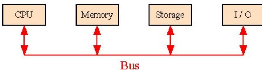
Data travels to and from all the computer's components via this "data highway". Though the bus seldom gets much attention when shopping for computers, it has a tremendous impact on the performance of the computer. Just like CPU's, bus designs have become more complex, and capable of operating at higher speeds.
