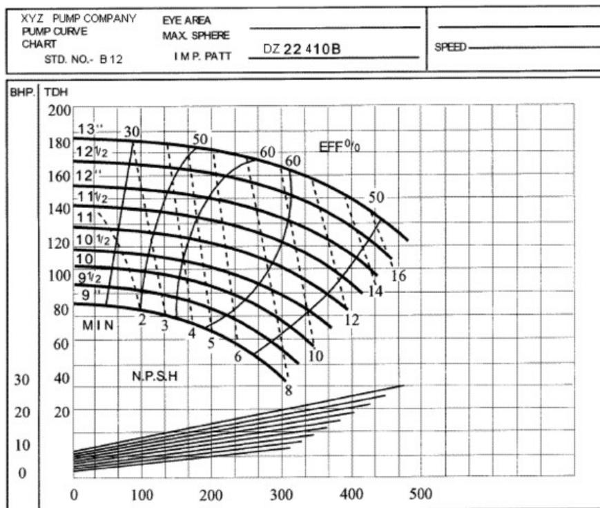
Lines of constant efficiency are plotted on manufacturer's pump performance curves as superimposed incomplete parabolic arcs generally opening in the positive direction. An rough estimate of the efficiency value using these plots is sometimes the best that can be accomplished from the pump performance curve.
