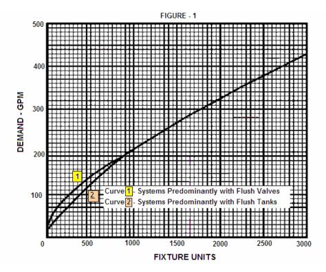
The figure above shows two separate curves; one for flush valve (curve 1) and other for flush tanks (curve 2). The curves show slight discrepancies from 0 to 1000 fixture units. The flush tank curve has slightly larger flowrate values within this range. The reason for different flowrate values has to do with sudden instantaneous draw rate of the flush valve. The
