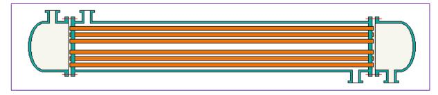
**BEM:** This is the same type of heat exchanger as above, but with **one tube pass**.
