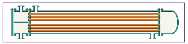
**AEM:** Channel with Removable Cover, One Pass Shell, Fixed Tubesheet Bonnet.
