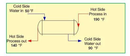
**Solution:** First calculate the **required heat transfer rate** for the above indicated light oil:
