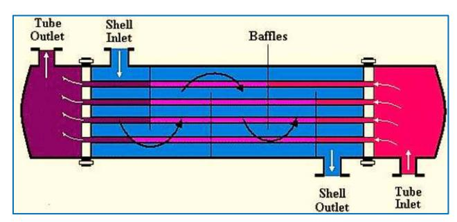
**Example 3:** Taking the shell and tube heat exchanger described in Example 1, how many tubes of **3.0-inch diameter** and **10 ft length** should be used?
