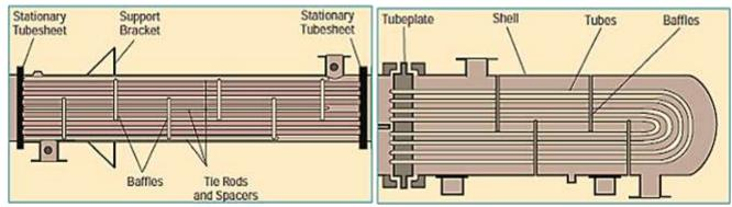
a) Fixed-tube Sheet Heat Exchanger.
