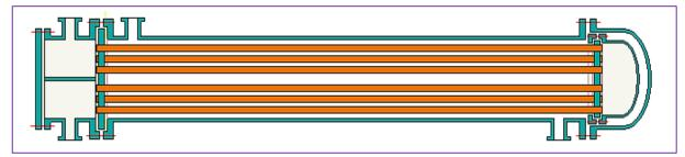
AES: Channel and Removable Cover, One Pass Shell, Floating Head with Backing Device.
