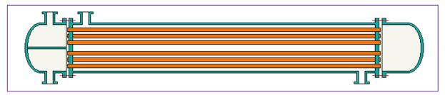
**BEM:** Bonnet (Integral Cover), One Pass Shell, Fixed Tubesheet Bonnet.
