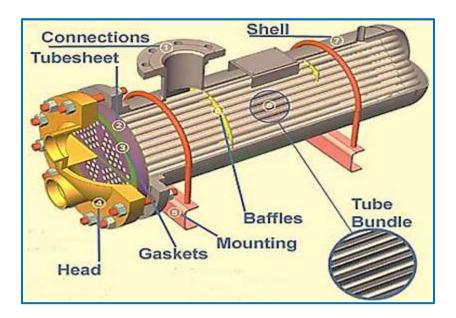
The optimum thermal design of a shell and tube heat exchanger involves the consideration of many interacting design parameters, which can be summarized as follows:
