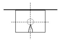
ASME BTH-1 (Ref. 4) refers to this failure as single plane fracture failure and provides an alternate method for calculating the tensile strength based on beyond the pin hole section:
