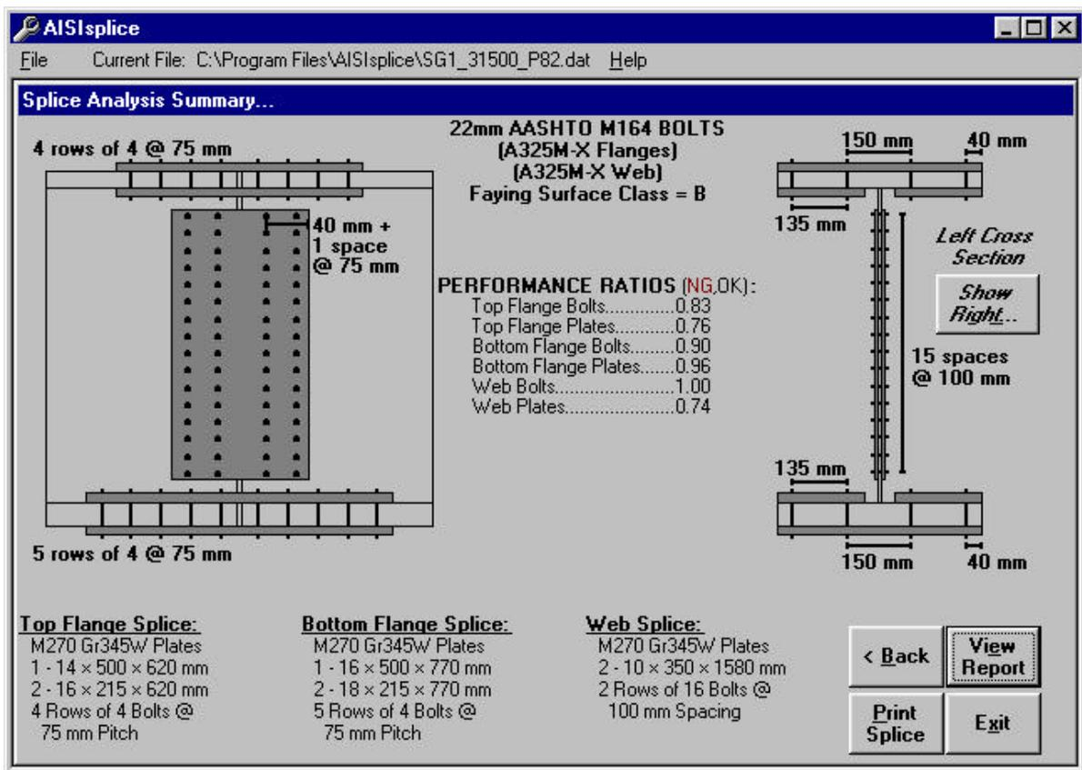
The Splice Analysis Summary screen includes all components of the Splice Design Summary screen, with the exception of the **Adjust Design** button (since an analysis is performed instead of design, thus the **Back** button may be used). The software also informs the user of any given spacing which does not satisfy the provisions of AASHTO 6.13.2.6.
