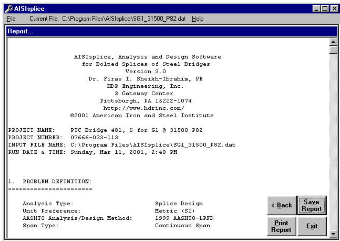
The report generated during the software execution can be viewed by clicking the **View Report** button on the graphical output screen. Once the Report screen is displayed, the user may use the scrollbar on the right of the Report screen, to easily view and navigate through the report.
