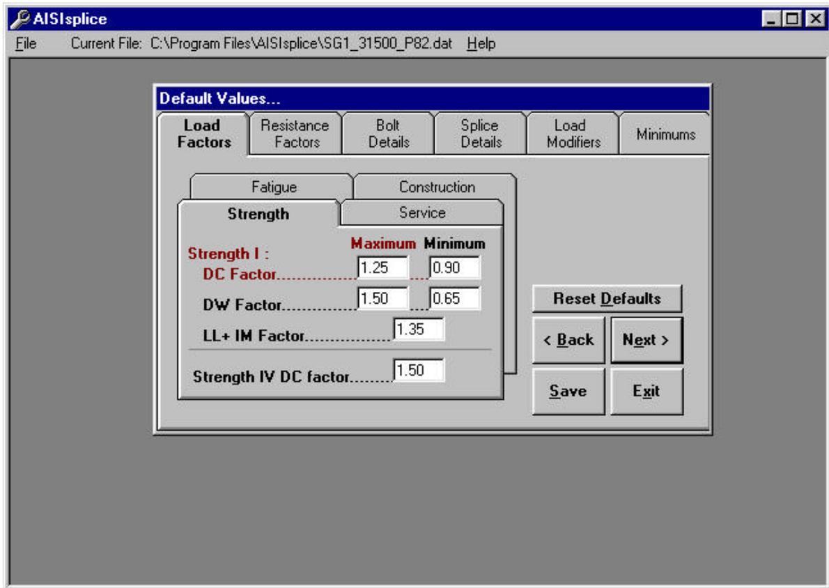
Access this tab to alter load factors for the construction, fatigue, service, and strength limit states. System defaults are taken from AASHTO 3.4.1 and 3.4.2. Maximum load factors must be greater than minimum load factors and less than 3.0 (selected arbitrarily), while minimum load factors may not be less than zero. In order to conservatively neglect wearing surface loads which oppose the live load moment, the user may elect to use a minimum wearing surface factor, DW, equal to zero.
