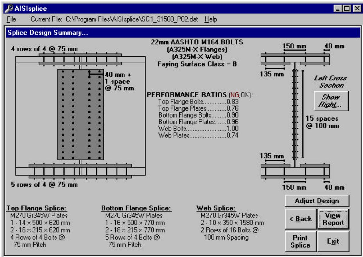
When designing a splice, the Splice Design Summary screen appears. This screen contains graphical output of splice details, required filler plates and their locations, girder cross sections and elevation views, properties of the flange and web connection bolts, faying surface class, and performance ratios.
