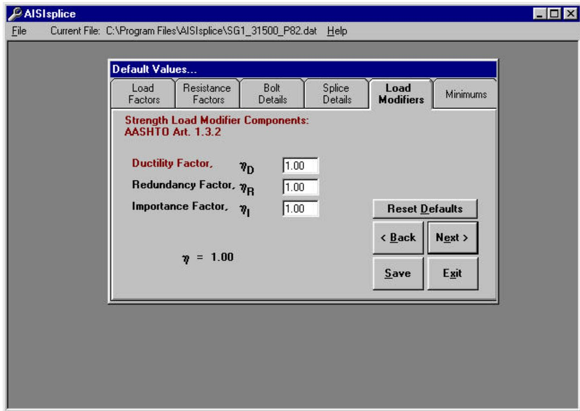
The value for the load modifier is dependent on factors relating to component and connection ductility, member redundancy, and operational importance of the bridge. The software default value for any load modifier is 1.0.
