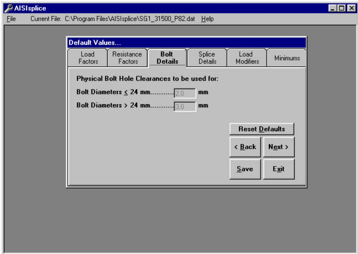
The **Bolt Details** tab shows the user the bolt hole clearances used (shown only for the SI units system).
