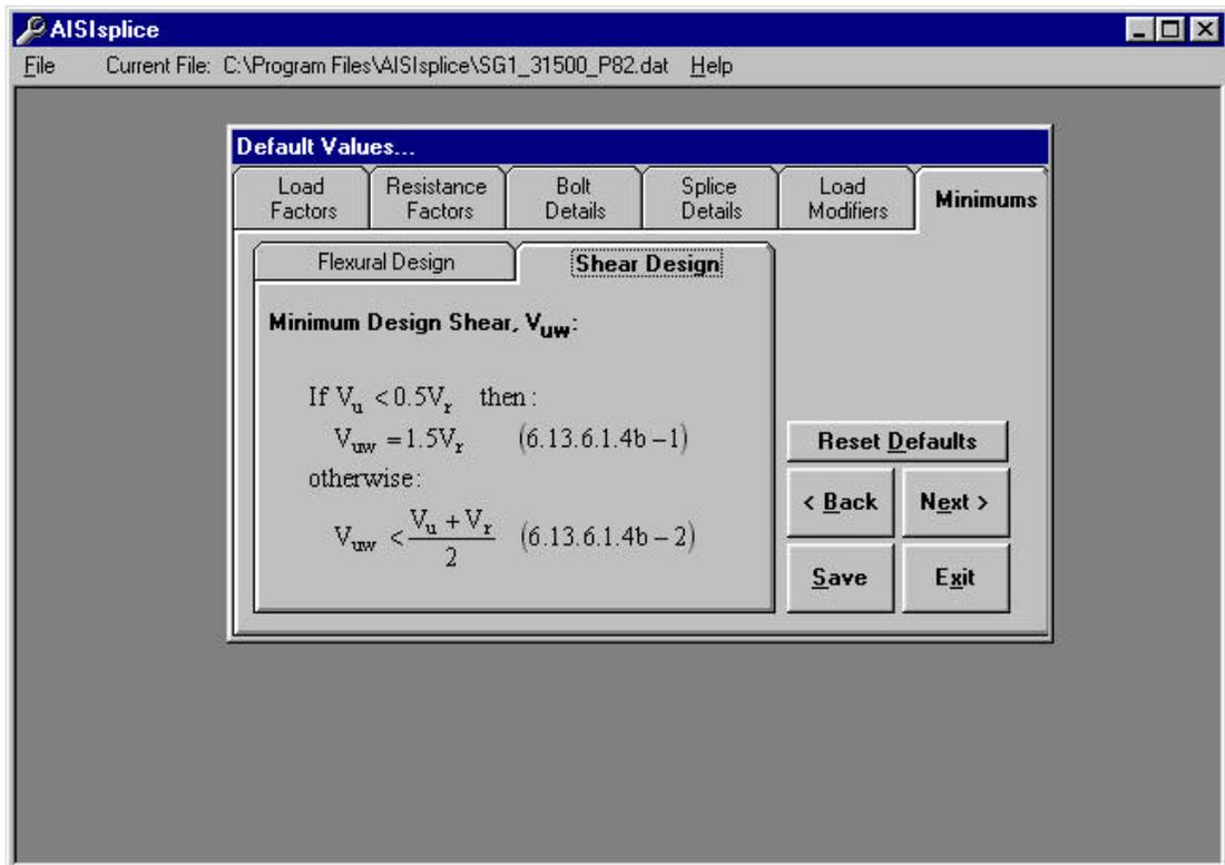
In order to comply with AASHTO 6.13.6.1.4c and 6.13.6.1.4b, flexural and shear design minimums should be used to further proportion flange and web design forces. The software applies flexural and shear design minimums, with respect to the **1999** Interim to the AASHTO LRFD Specifications.
