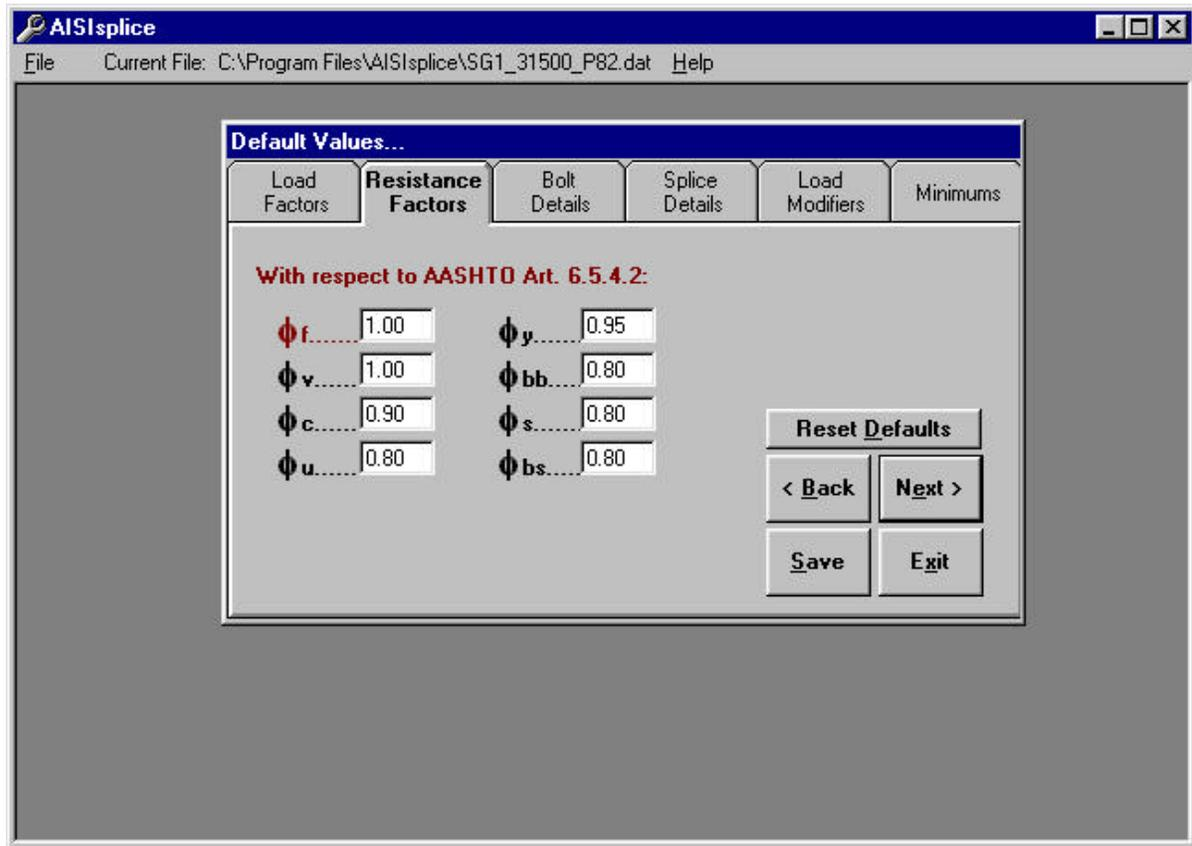
Click this tab in order to modify resistance factors (such as those for tensile gross section yielding, plate bearing, block shear, etc.) given by AASHTO 6.5.4.2. Resistance factors which are less than 0.50 or greater than 1.0 will not be accepted by the software.
