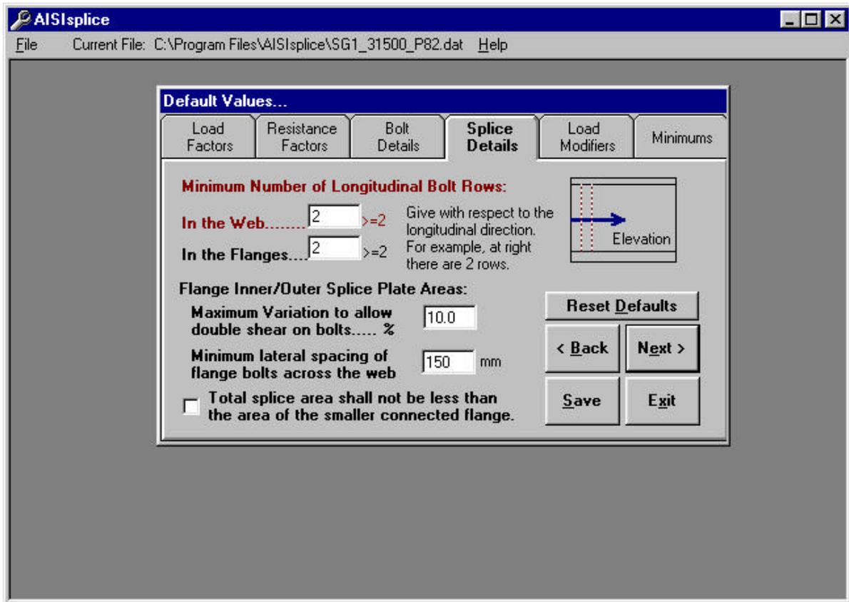
Click the **Splice Details** tab to set minimum limits on the number of required longitudinal flange and web bolt rows (the software will not accept values less than 2).
